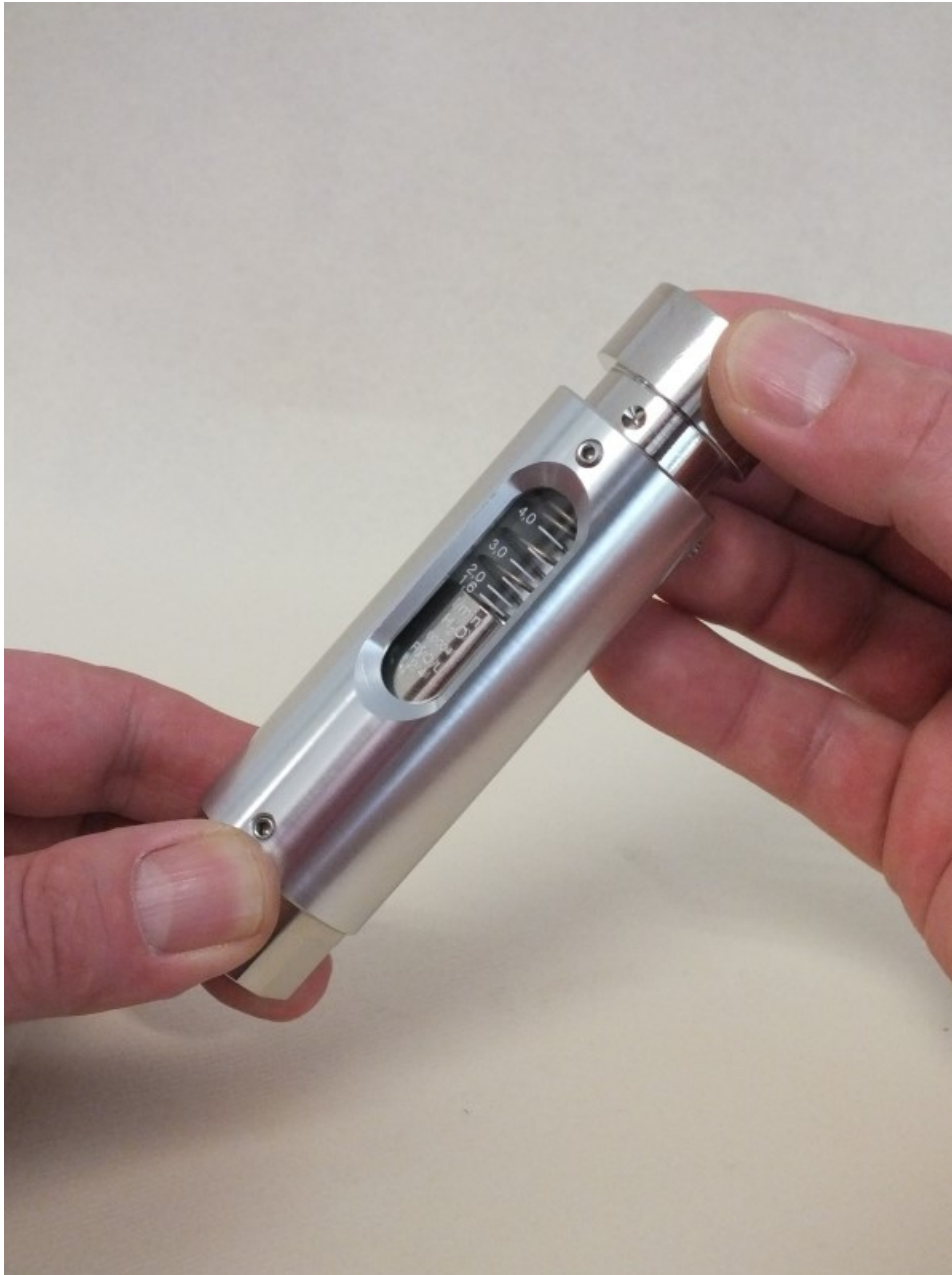
Fig. 49: Position the process connection (outlet)
