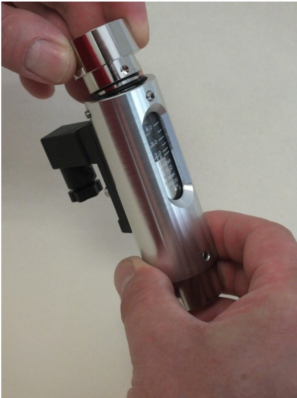
Fig. 35: Remove the process connection (outlet)
