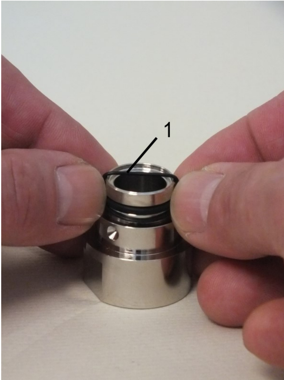
Fig. 40: O-ring (glass buffer)
