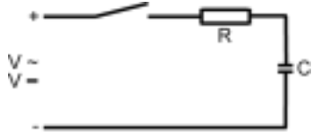
Fig. 28: Protective measure against capacitive loads
