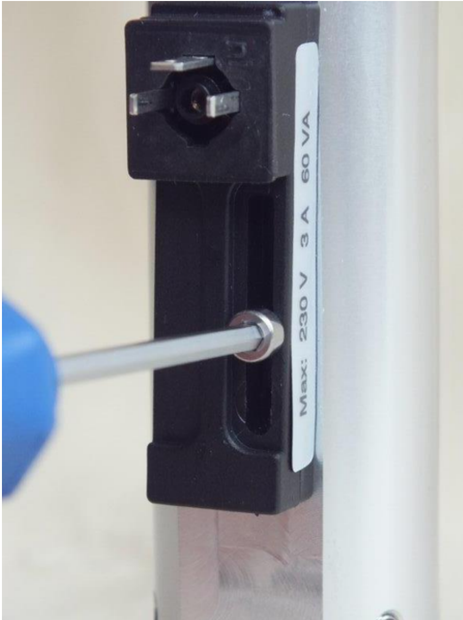
Fig. 31: Loosen set screw
