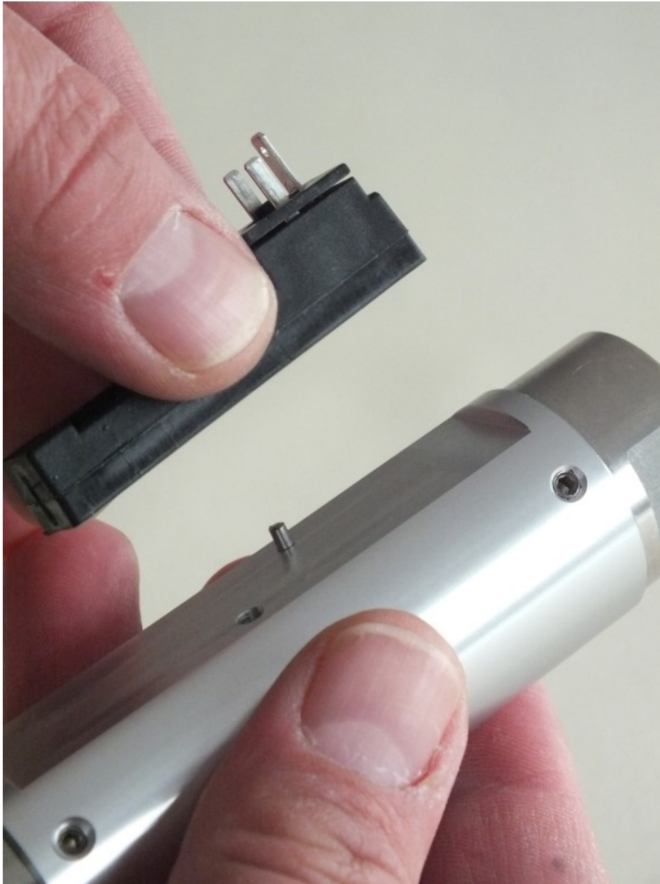
Fig. 55: Remove switch contact
