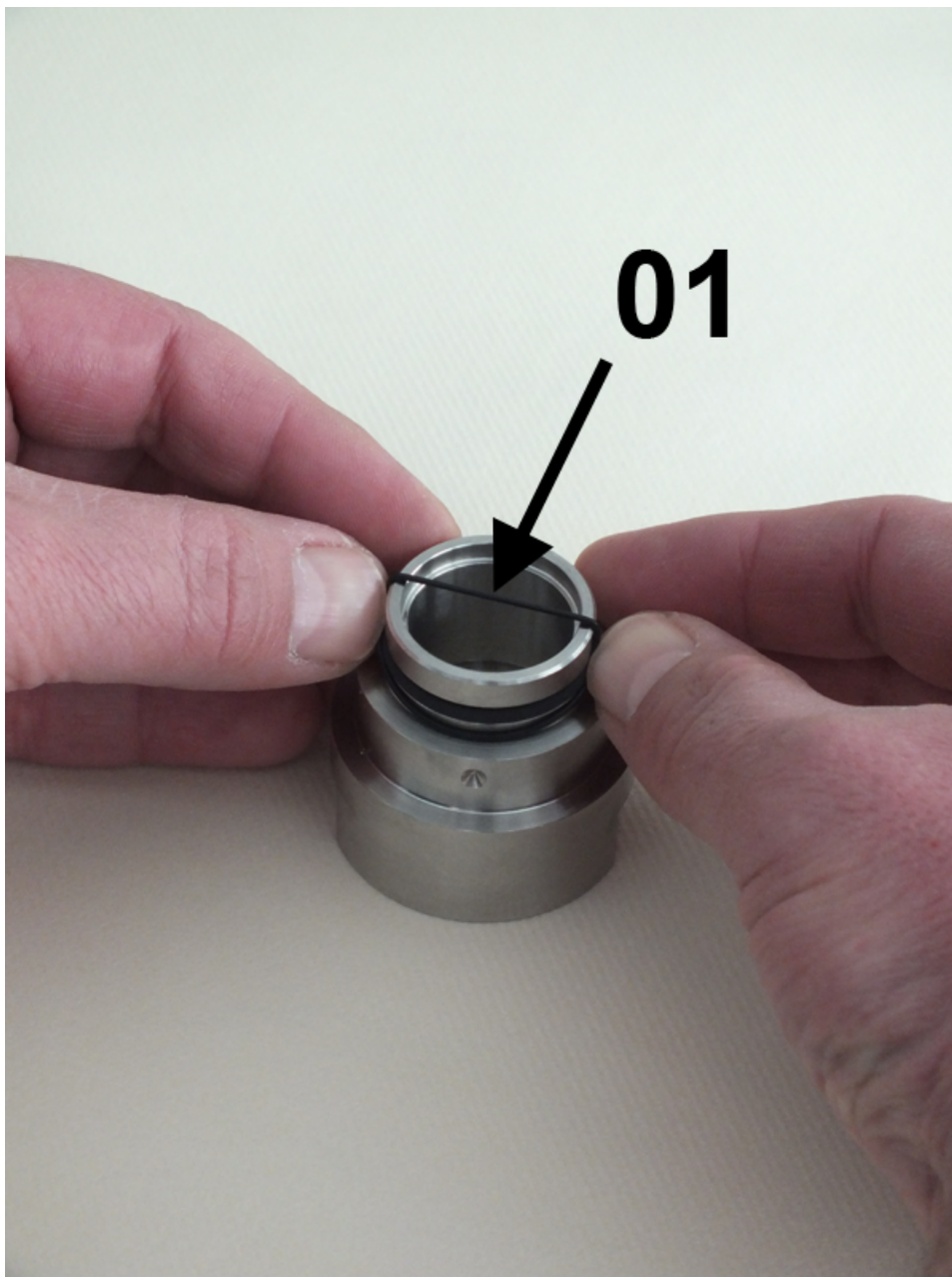
Fig. 41: O-ring (Glass buffer)
