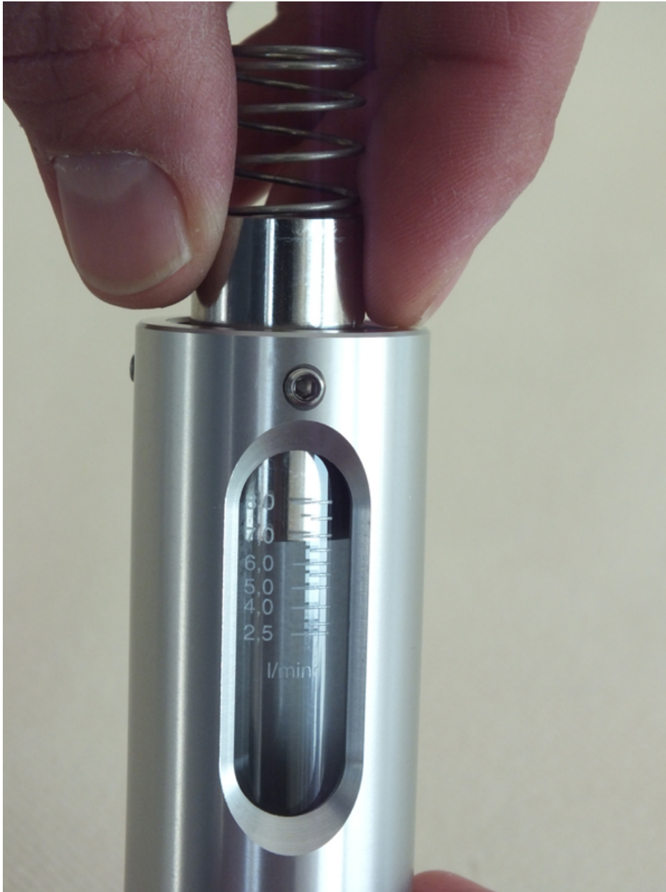
Fig. 49: Insert float and inner parts
