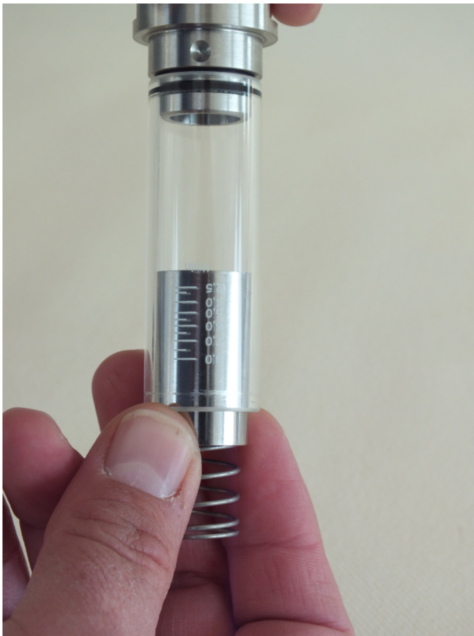
Fig. 39: Remove float, magnets and spring
