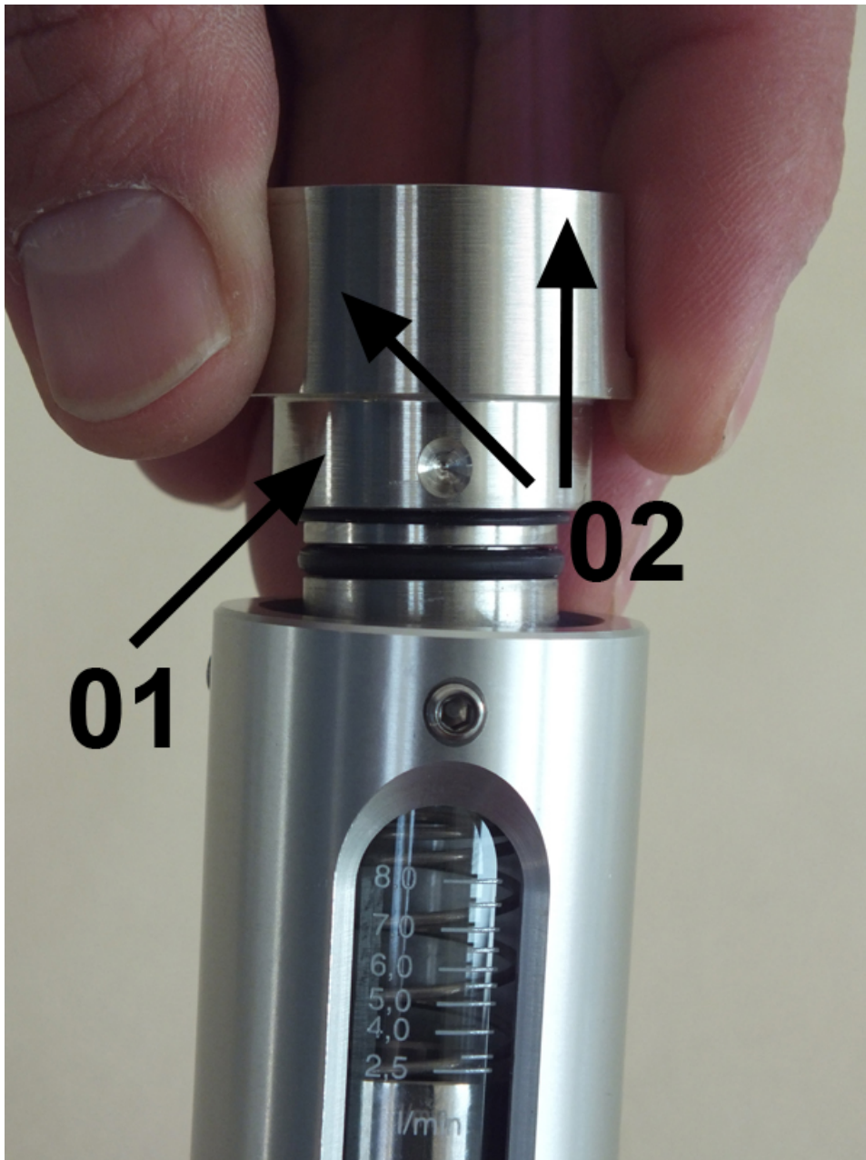
Fig. 50: Position process connection (outlet) in device housing
