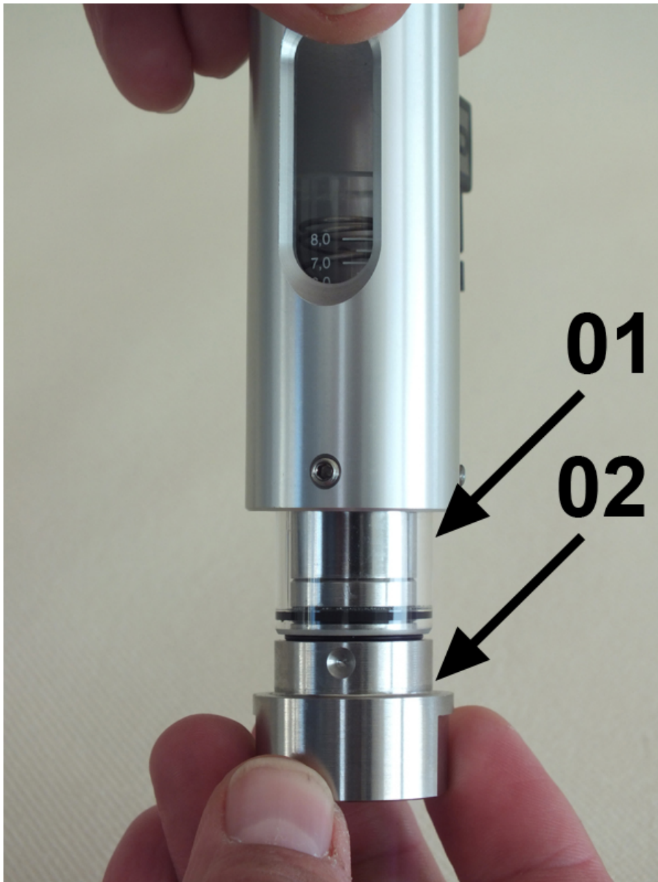
Fig. 38: Remove the inner section
