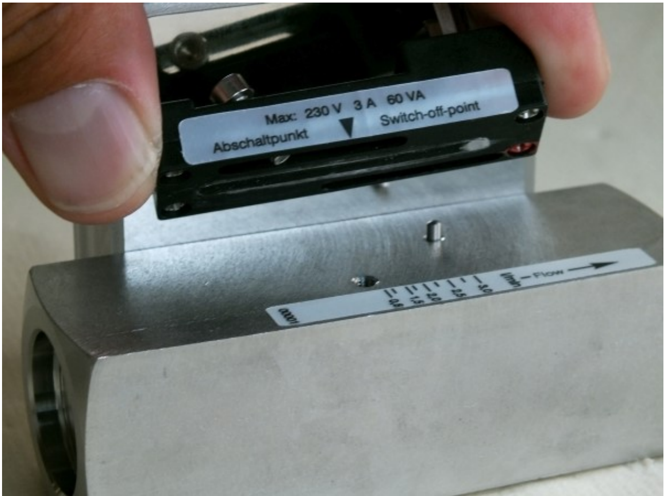
Fig. 70: Remove switch contact
