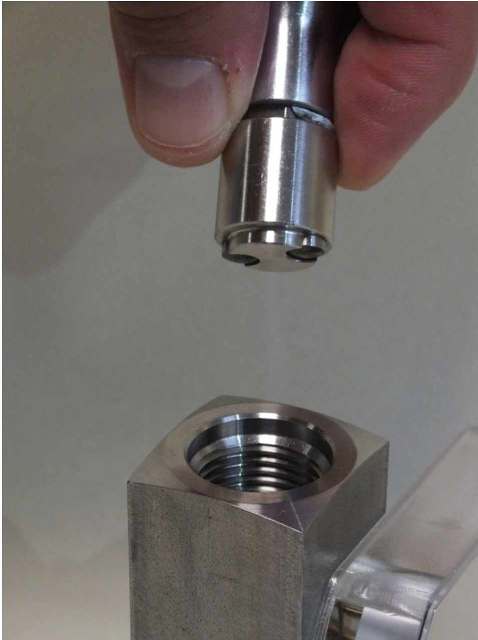
Fig. 44: Insert threaded ring insertion tool (outlet)
