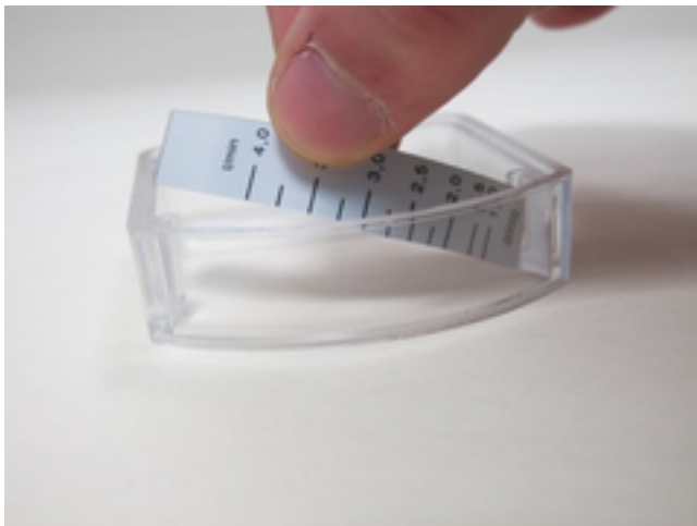
Fig. 40: Loosen the scale carrier
