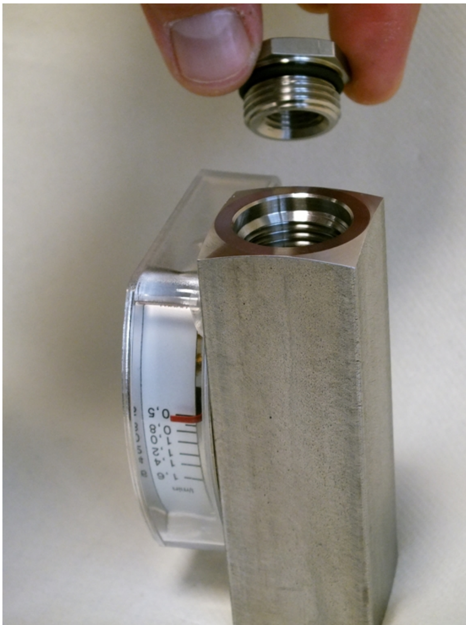
Fig. 50: Remove the process connection (inlet)
