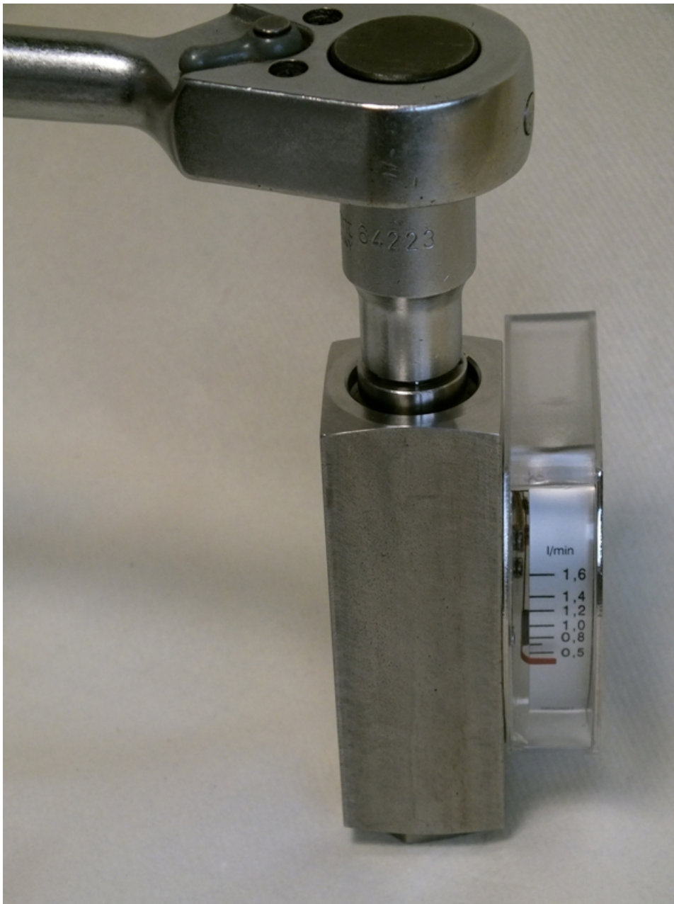
Fig. 45: Loosen threaded ring (outlet)
