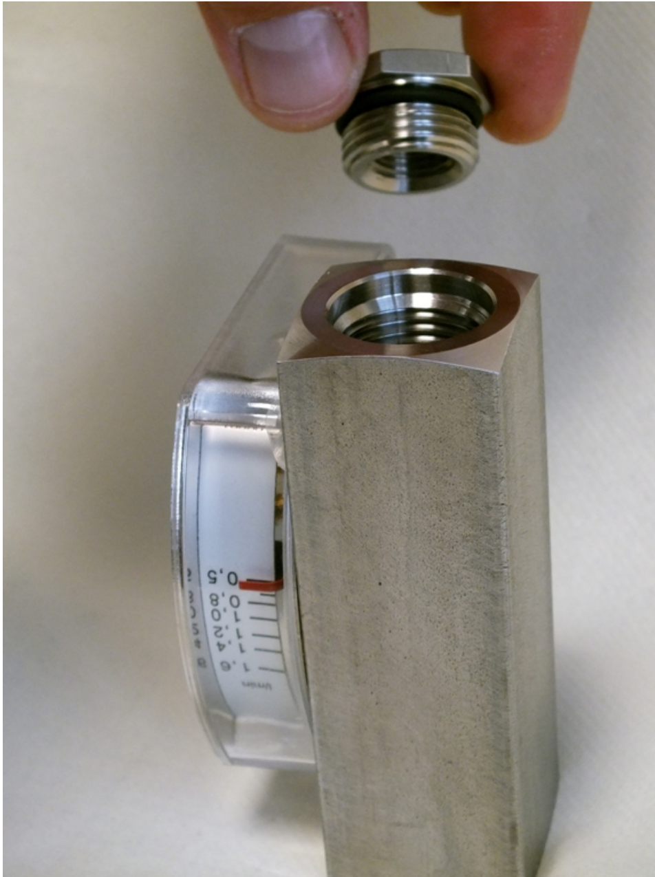
Fig. 53: Insert process connection (inlet)
