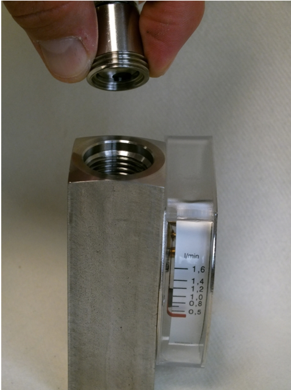
Fig. 46: Remove threaded ring (outlet)
