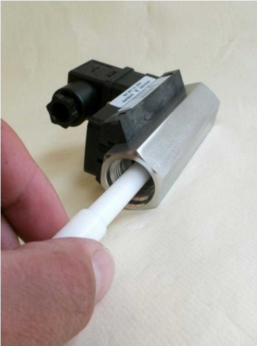
Fig. 47: Check for smooth operation
