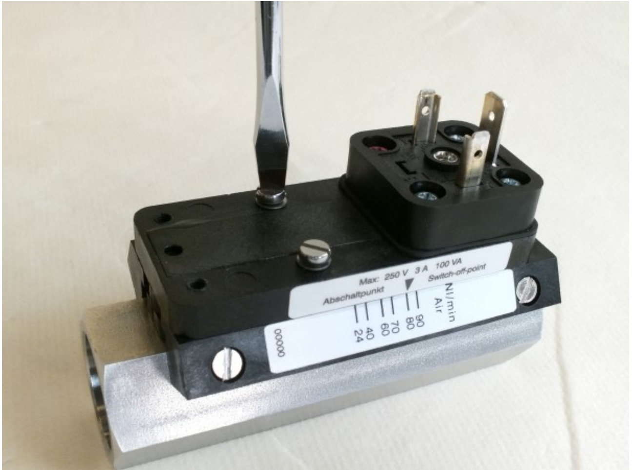
Fig. 50: Loosen set screws
