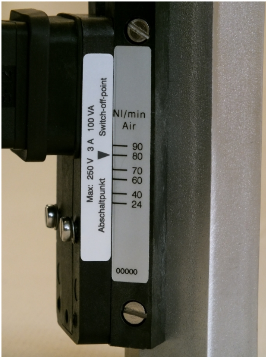
Fig. 4: Switch point adjustment scale RVM/U-L2 30x70
