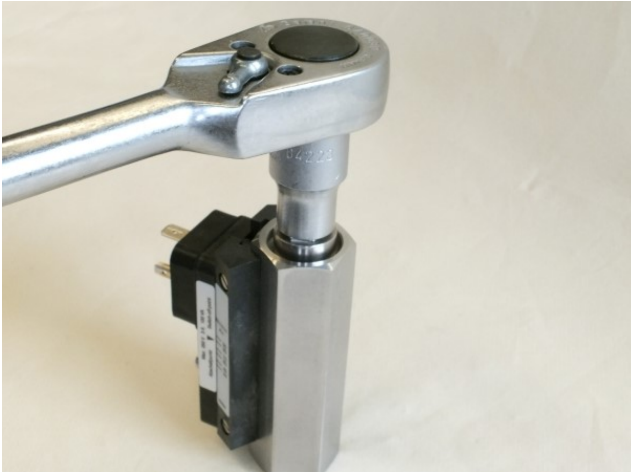
Fig. 39: Loosen threaded ring (outlet)
