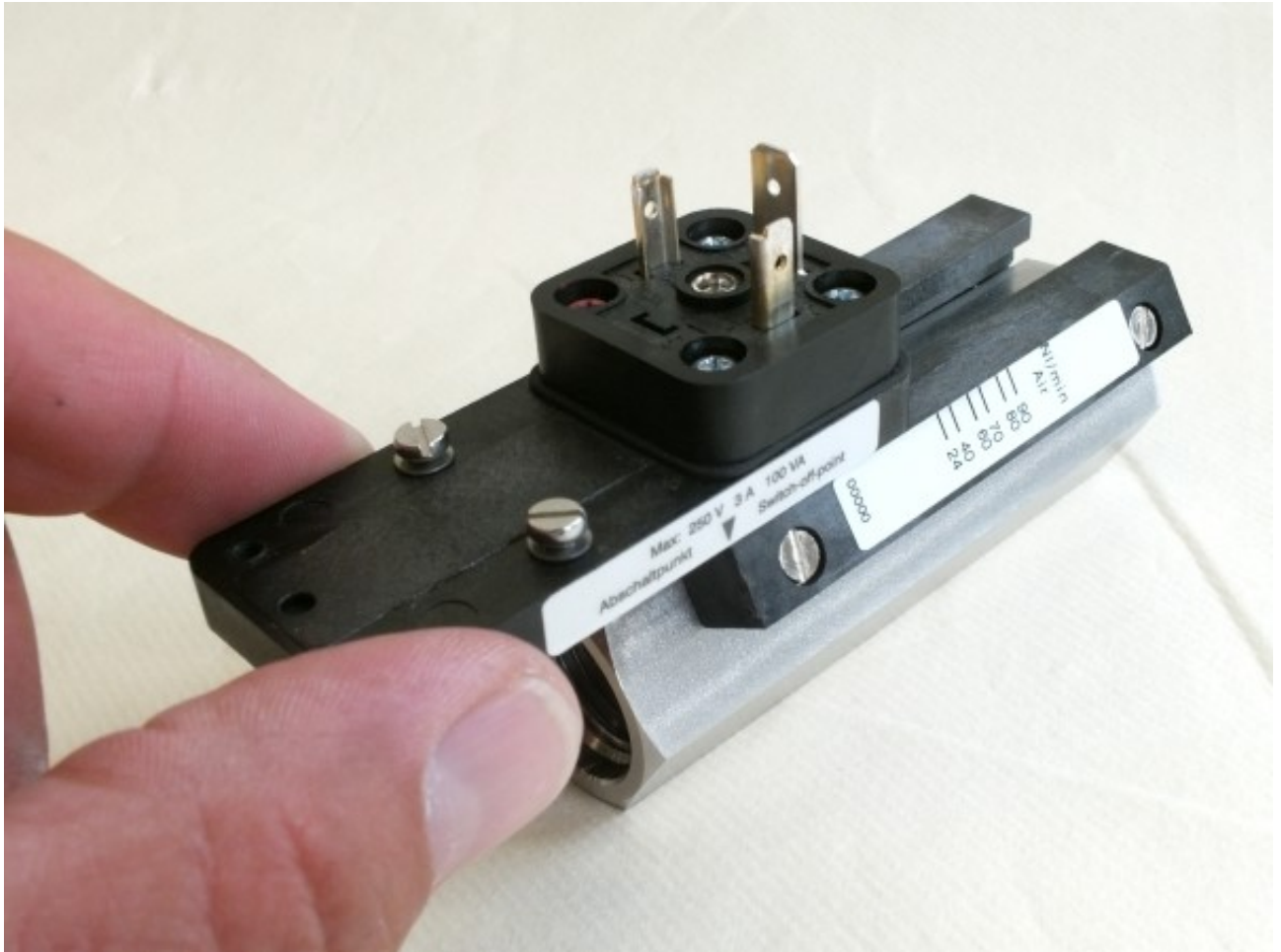
Fig. 51: Remove switch contact from guide rails
