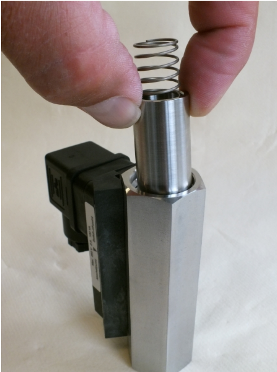
Fig. 44: Insert inner parts
