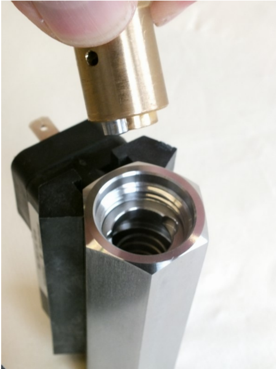
Fig. 38: Insert threaded ring insertion tool (outlet)
