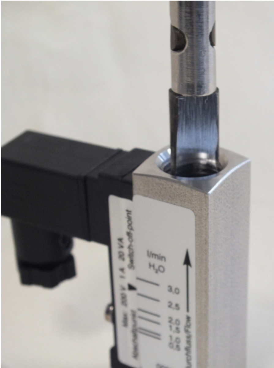
Fig. 36: Loosen threaded ring (outlet)
