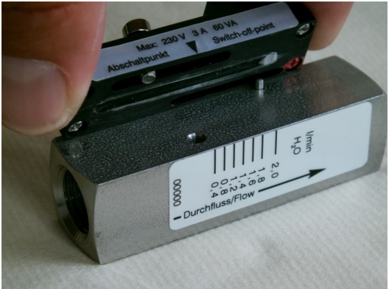
Fig. 53: Remove switch contact
