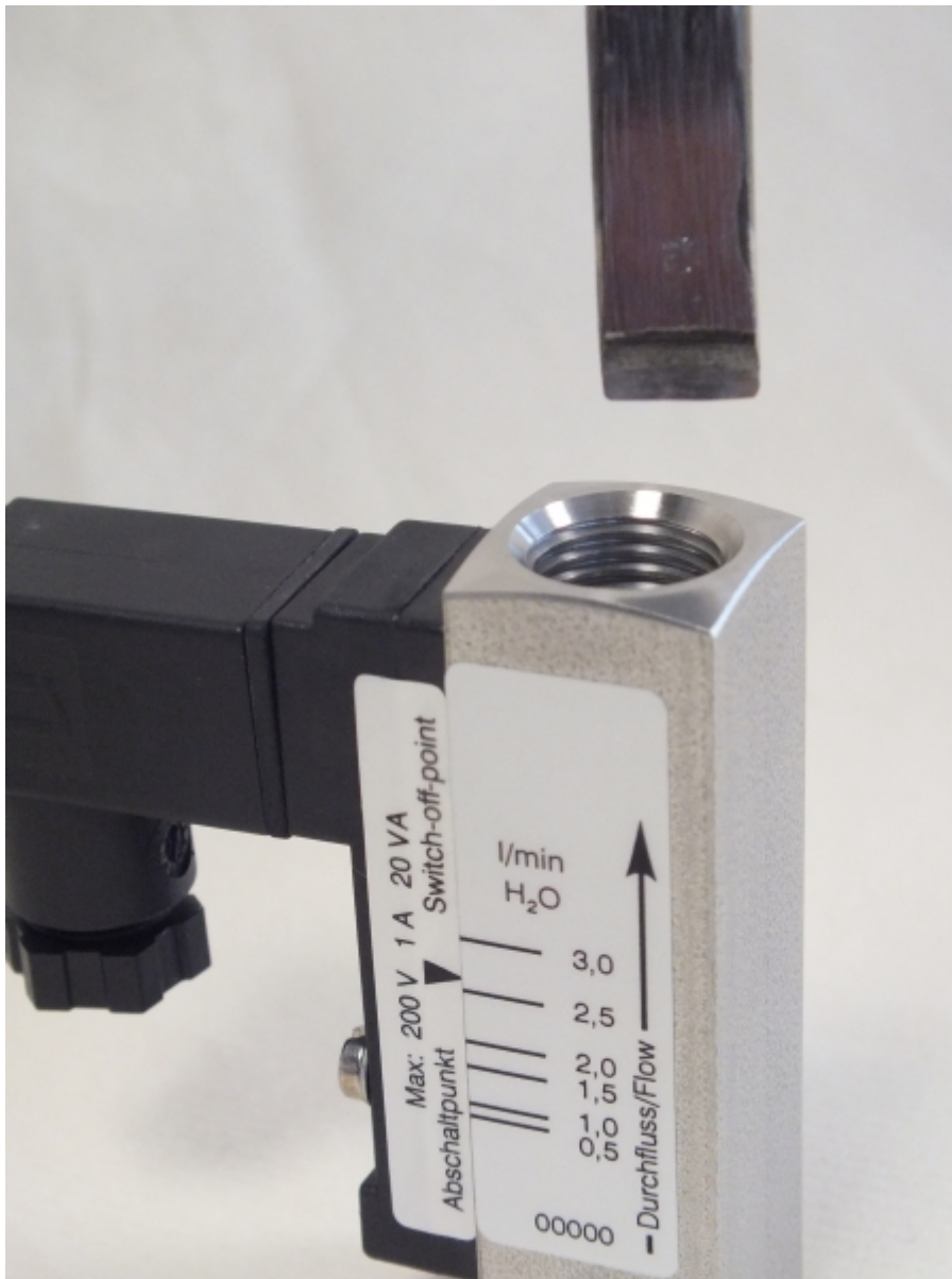
Fig. 35: Insert threaded ring insertion tool (outlet)
