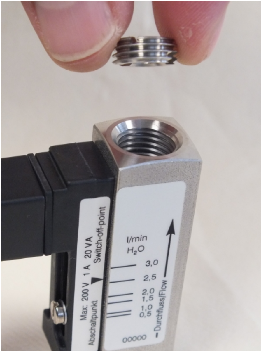
Fig. 37: Remove threaded ring (outlet)
