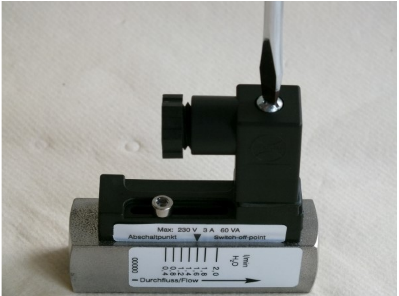
Fig. 50: Loosen female socket
