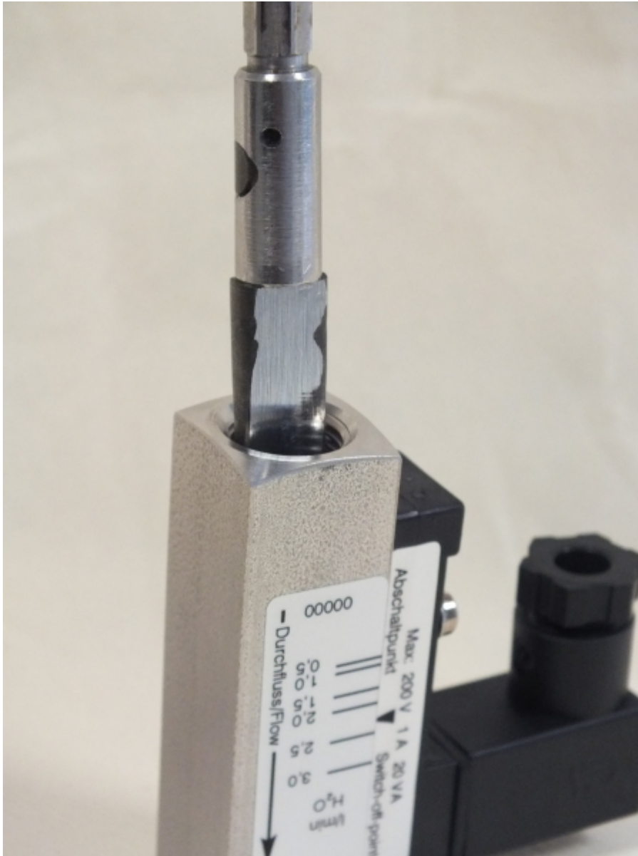
Fig. 41: Loosen threaded ring (inlet)
