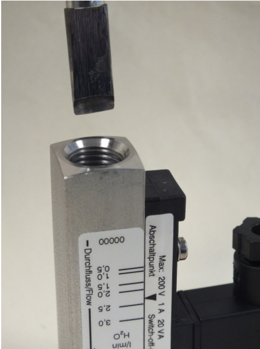
Fig. 40: Insert threaded ring insertion tool (inlet)
