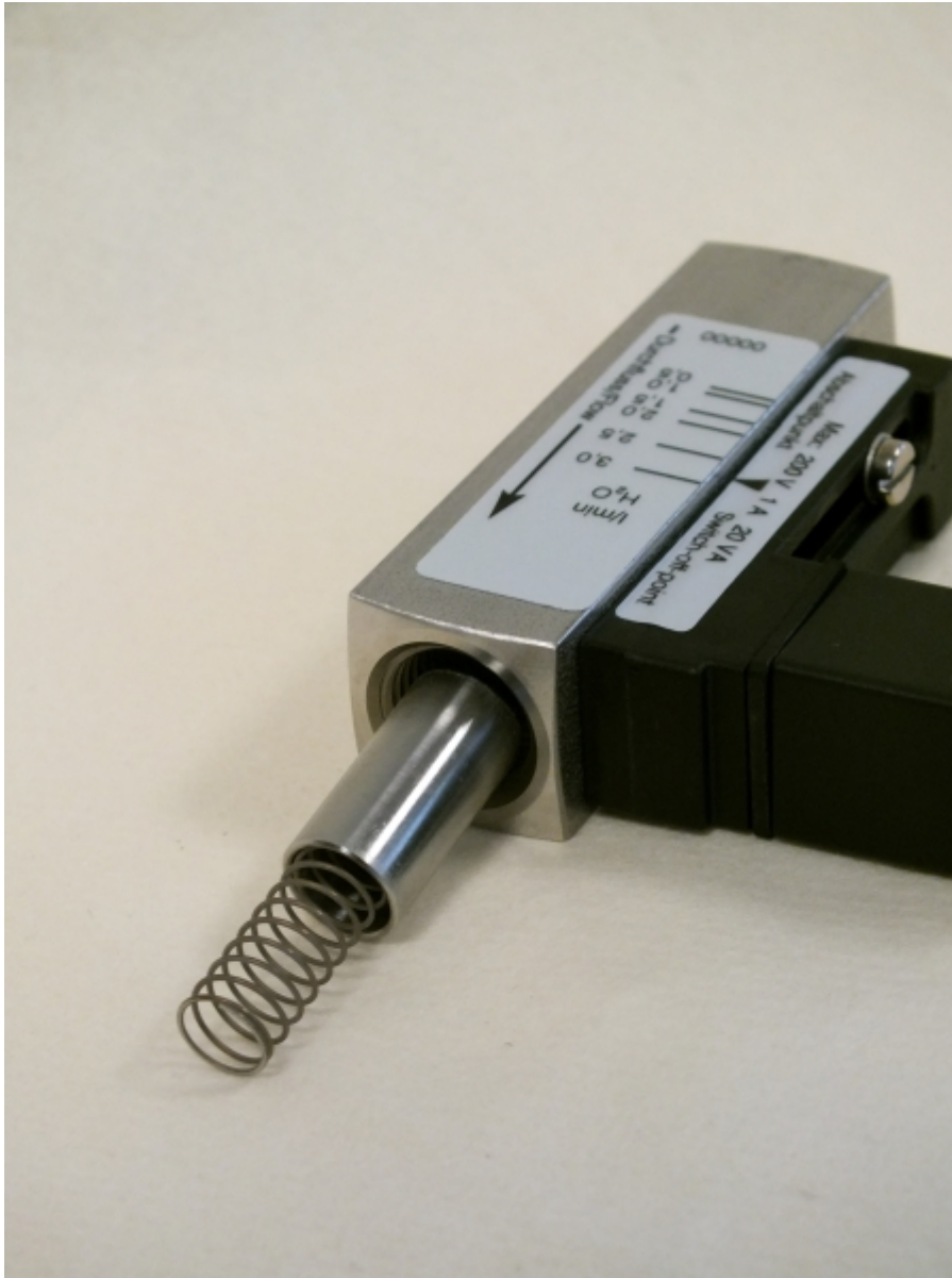
Fig. 38: Remove inner parts
