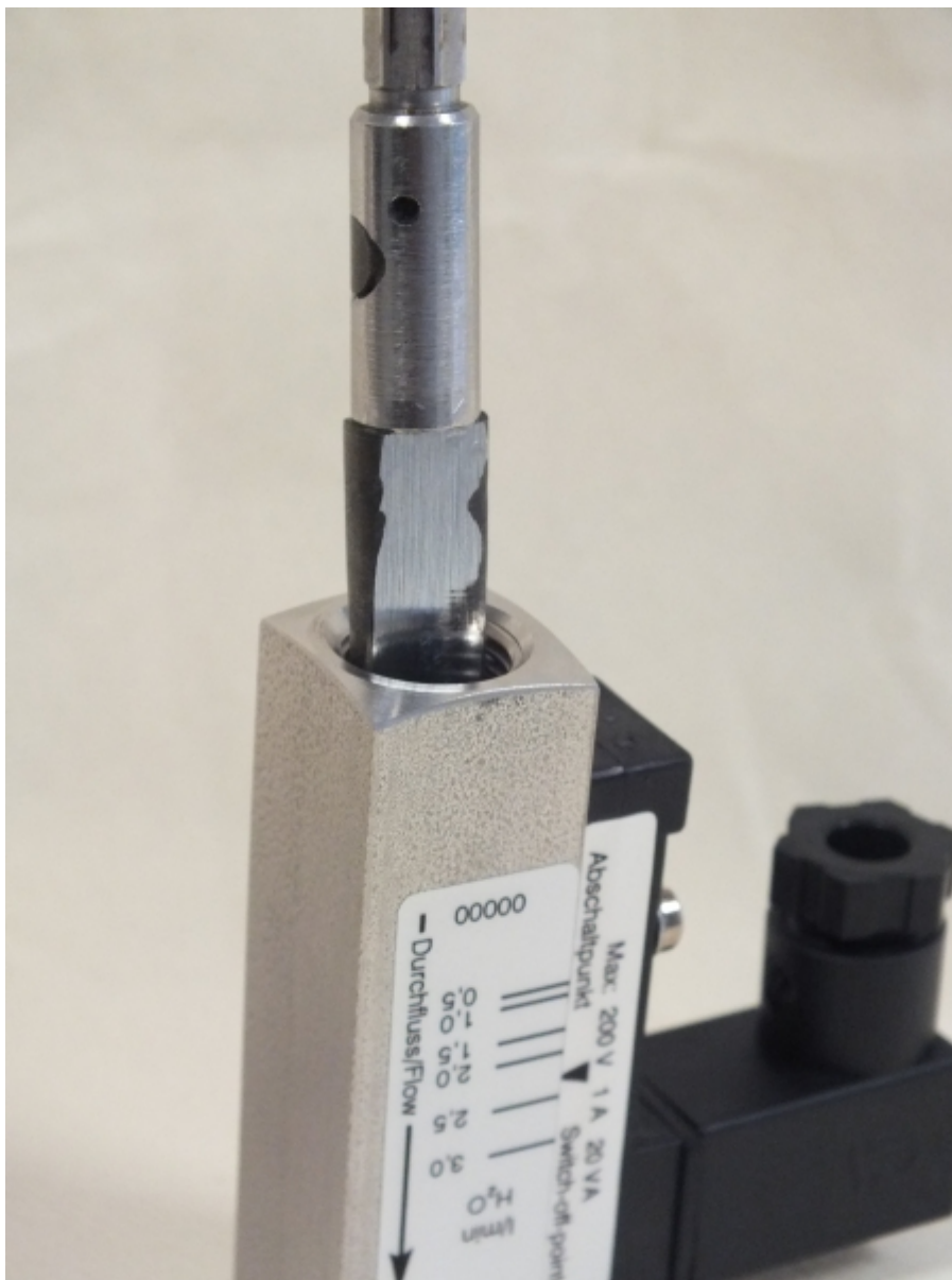
Fig. 44: Seat threaded ring (inlet)
