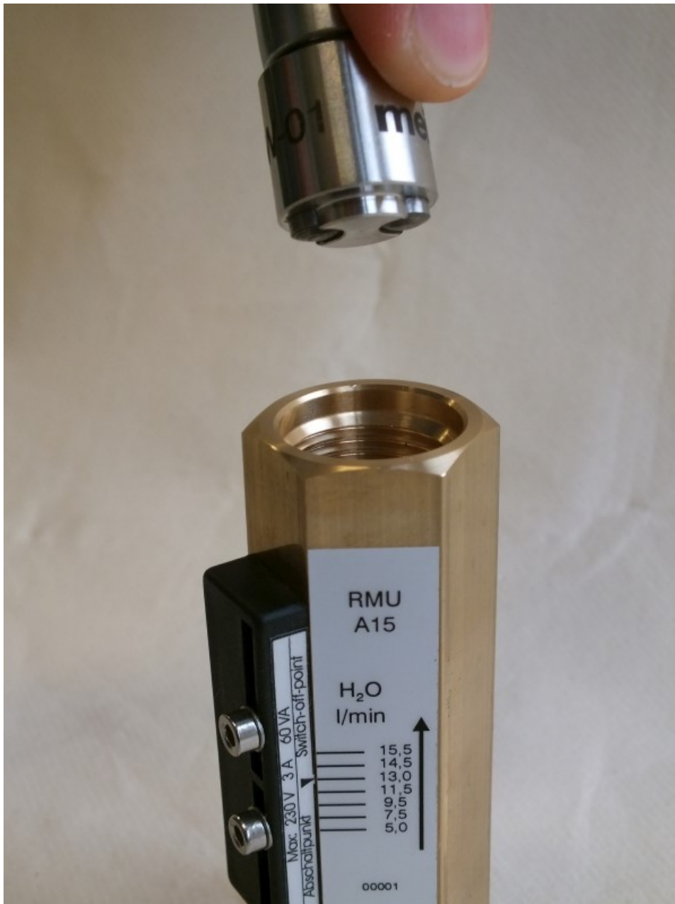
Fig. 22: Insert threaded ring insertion tool (outlet)
