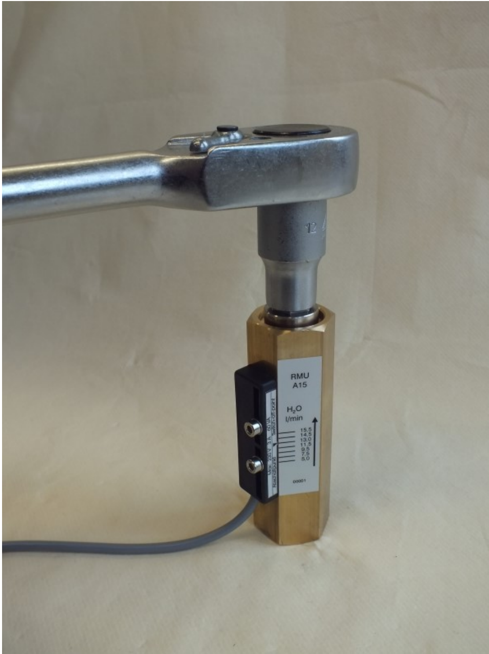
Fig. 23: Loosen threaded ring (outlet)
