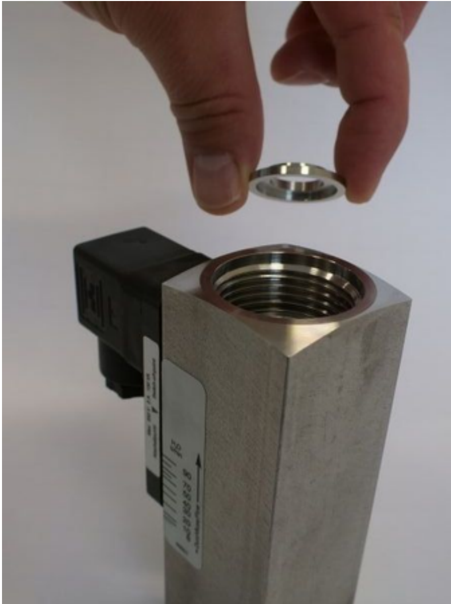
Fig. 43: Remove the centering disc (outlet)
