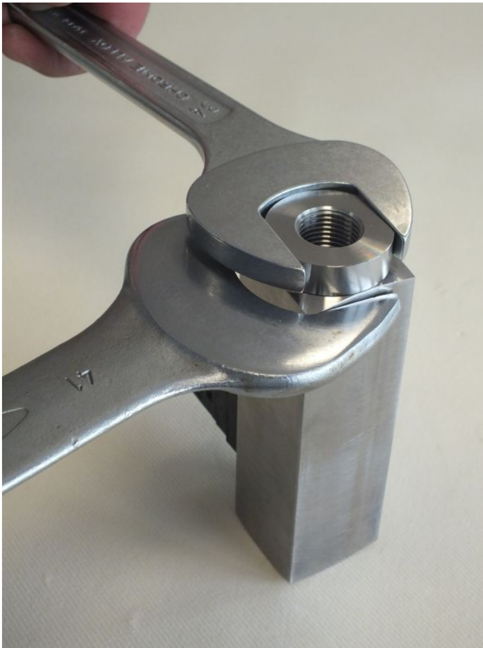
Fig. 51: Tighten process connection (inlet)
