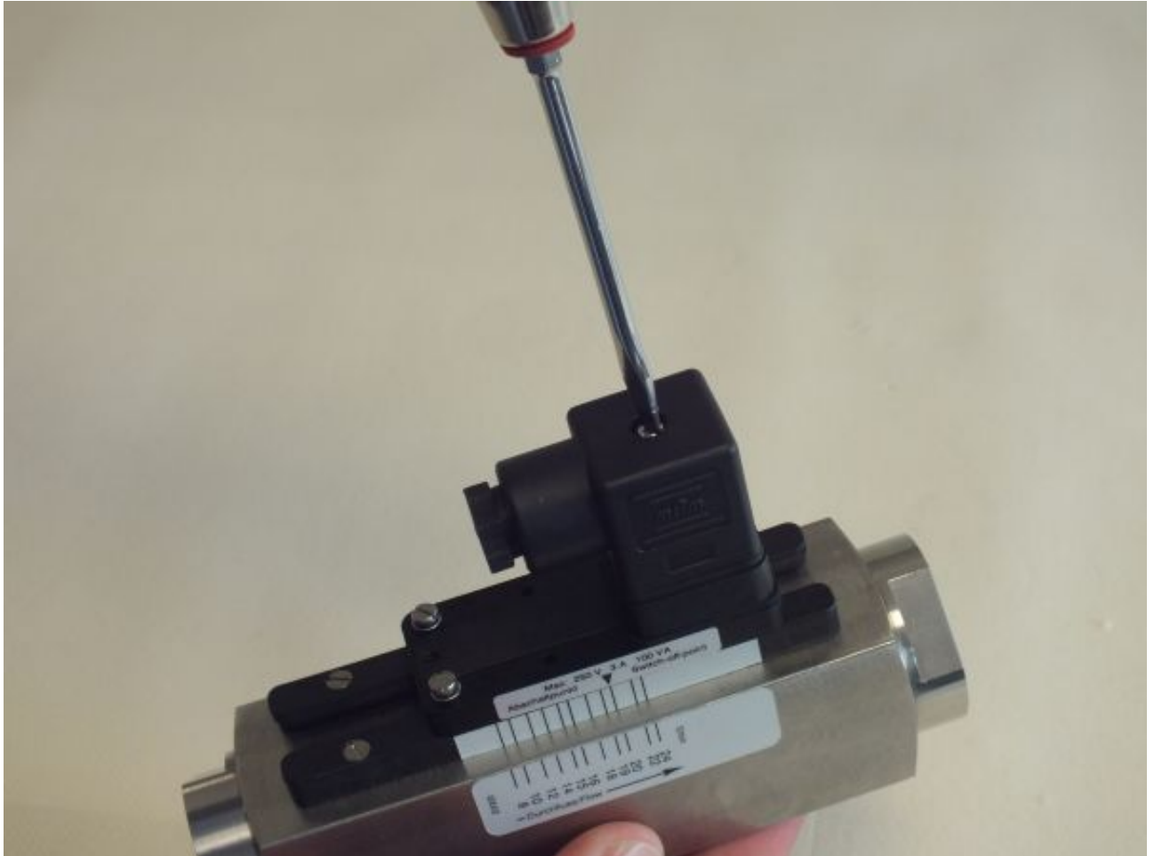
Fig. 58: Loosen female socket
