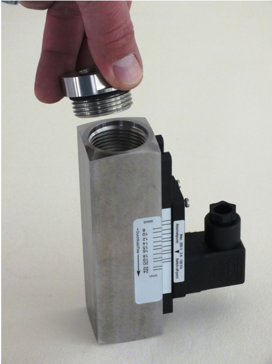
Fig. 47: Remove the process connection (inlet)
