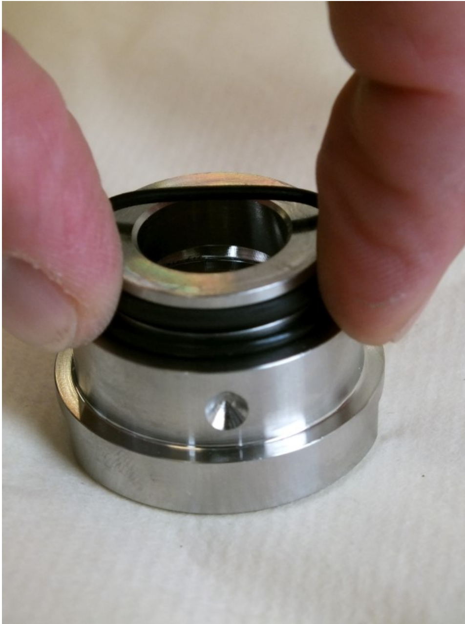
Fig. 48: O-ring (glass buffer)
