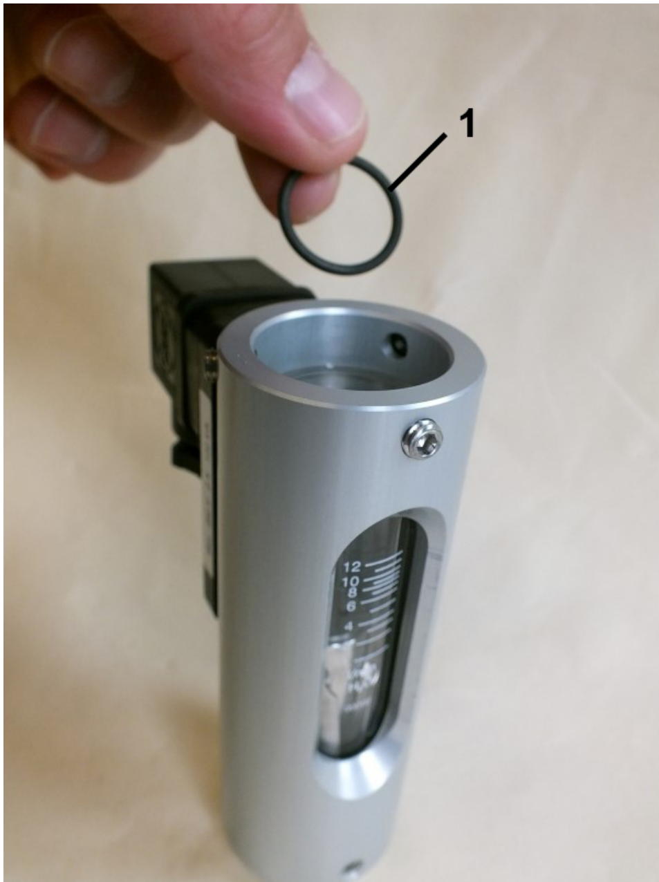
Fig. 43: Slot nozzle buffer O-ring
