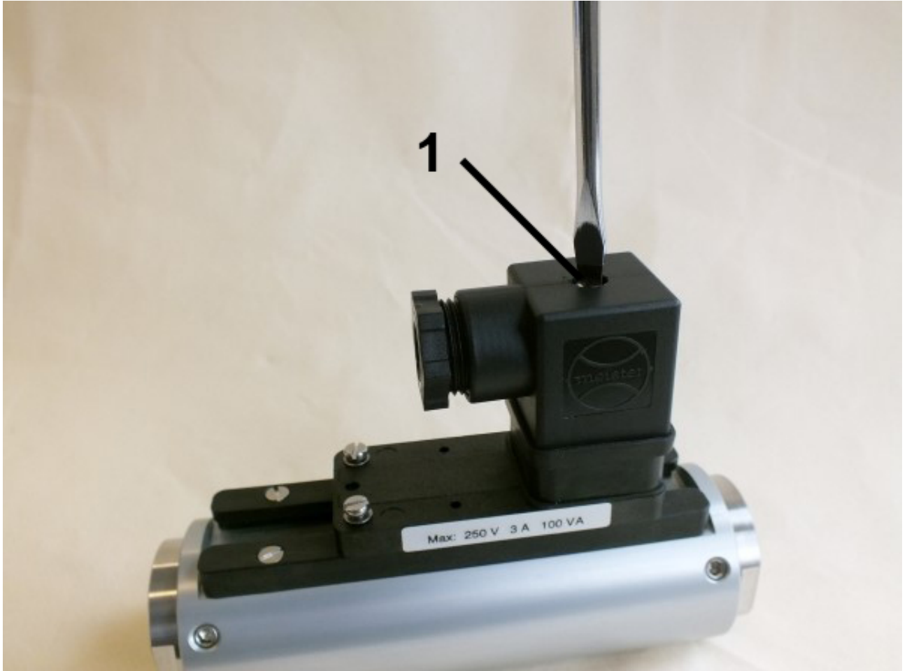
Fig. 63: Loosen female socket
