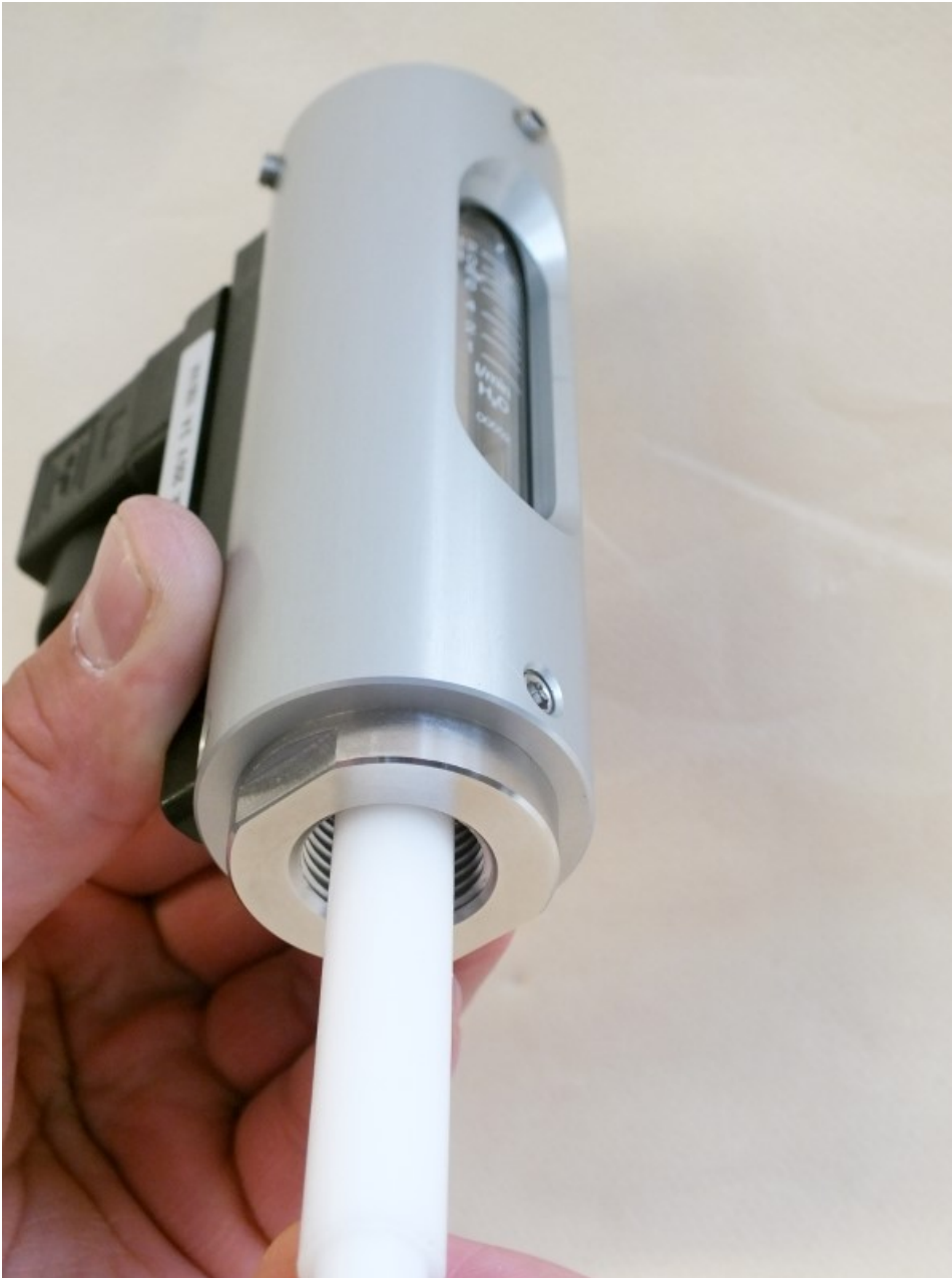
Fig. 62: Check for free movement
