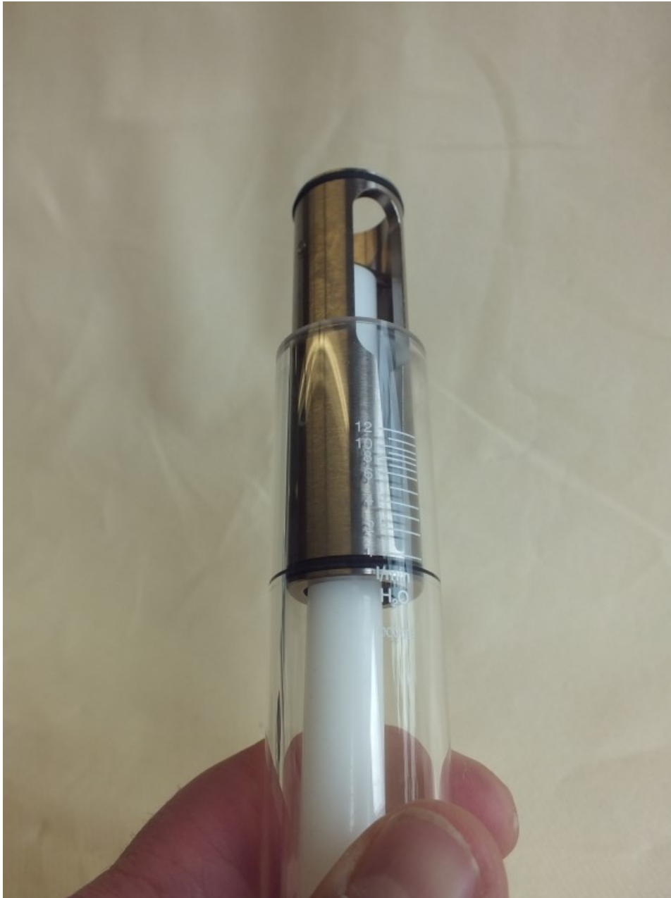
Fig. 46: Remove slot nozzle
