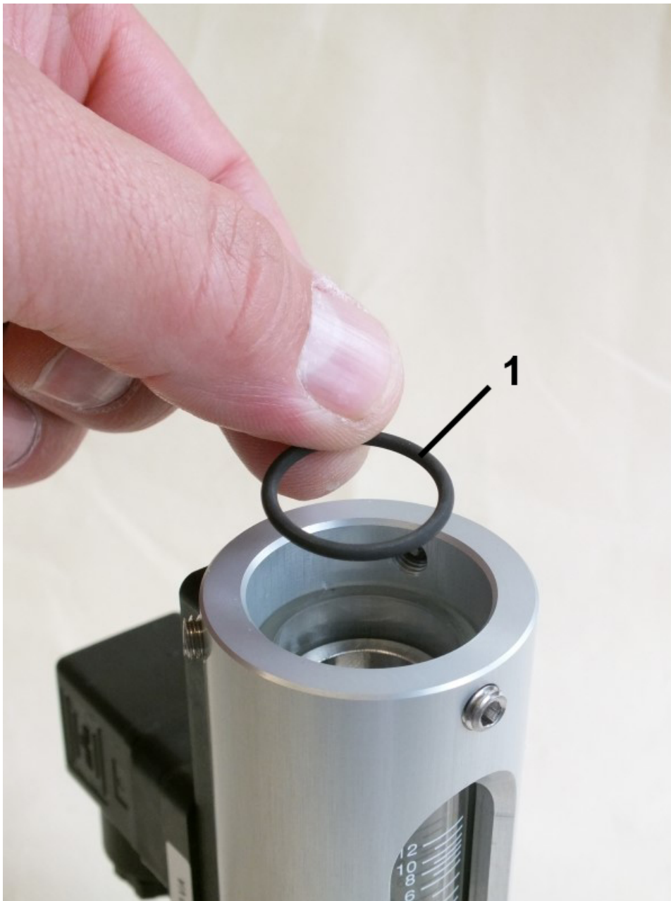
Fig. 59: O-ring, slot nozzle buffer
