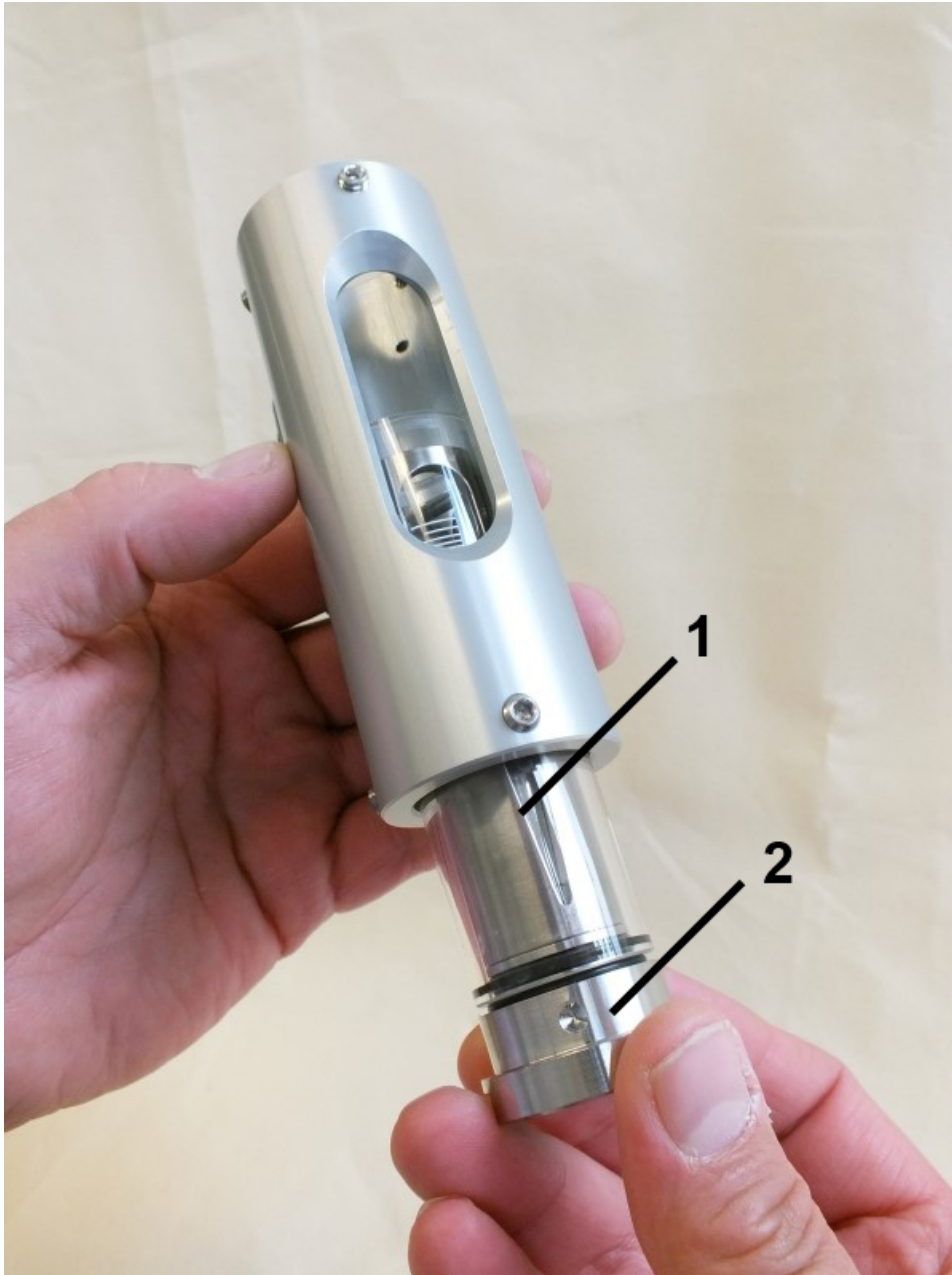
Fig. 45: Remove the inner section
