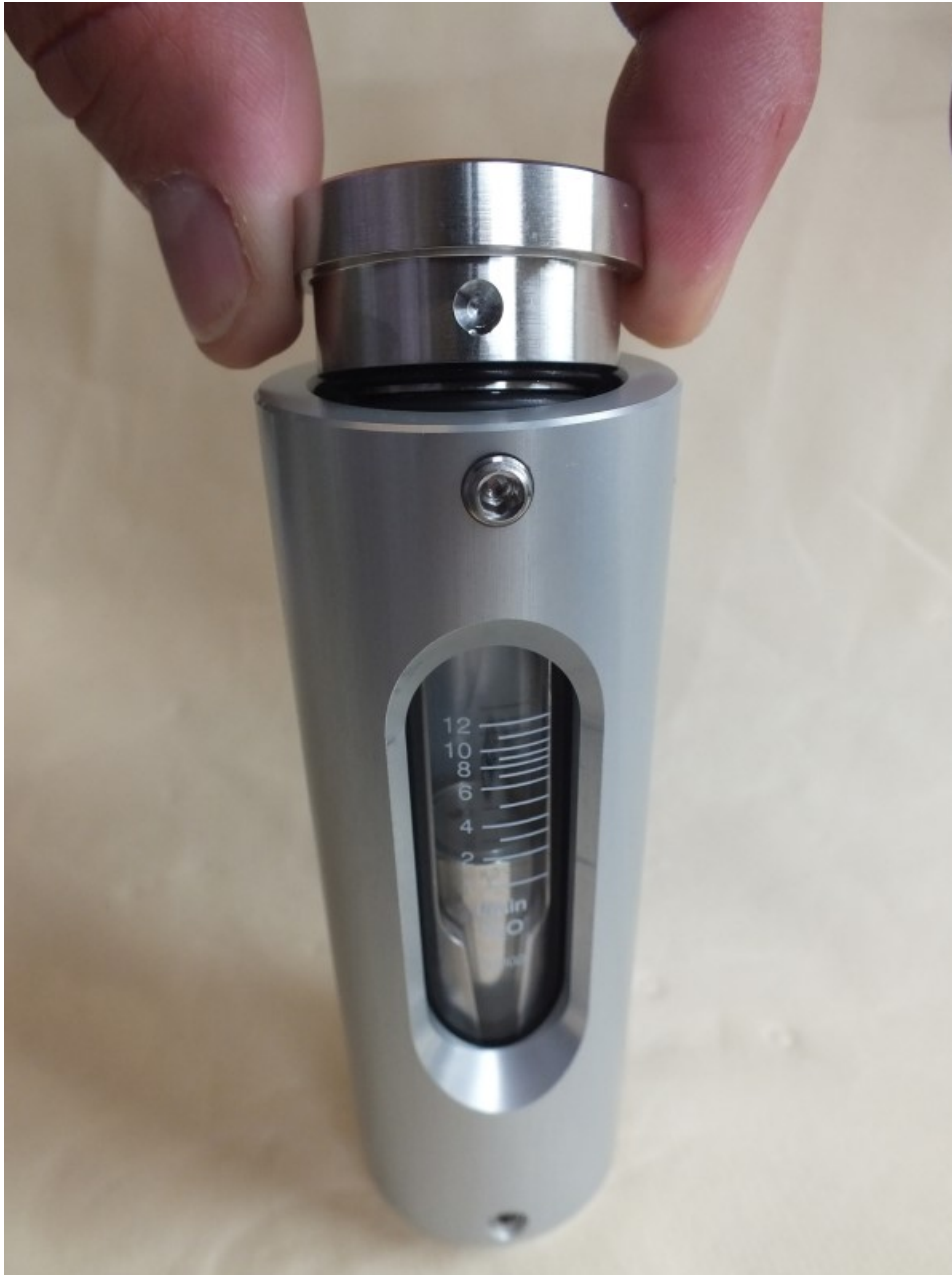
Fig. 42: Remove the process connection (outlet)
