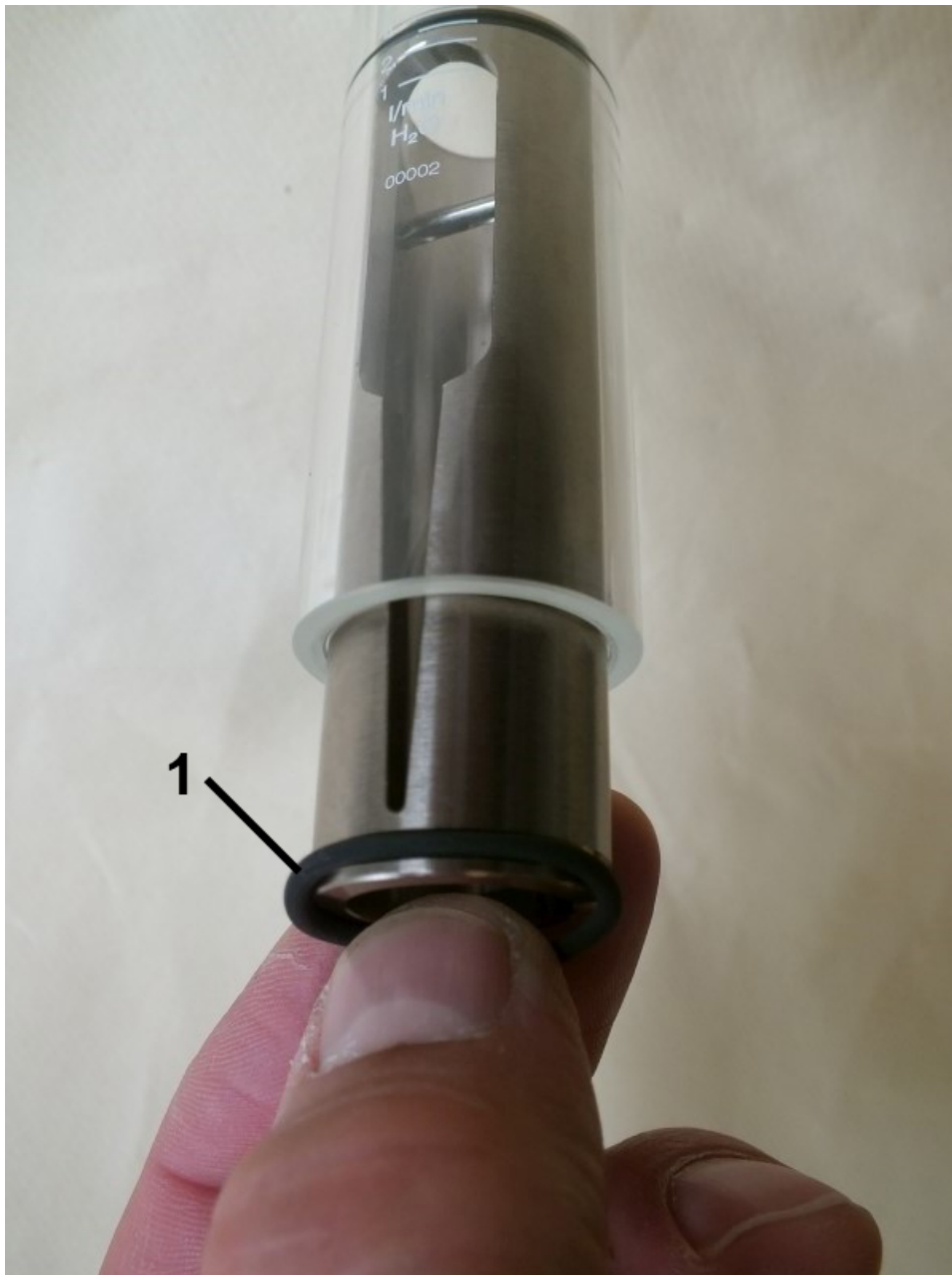
Fig. 52: Centering the slot nozzle
