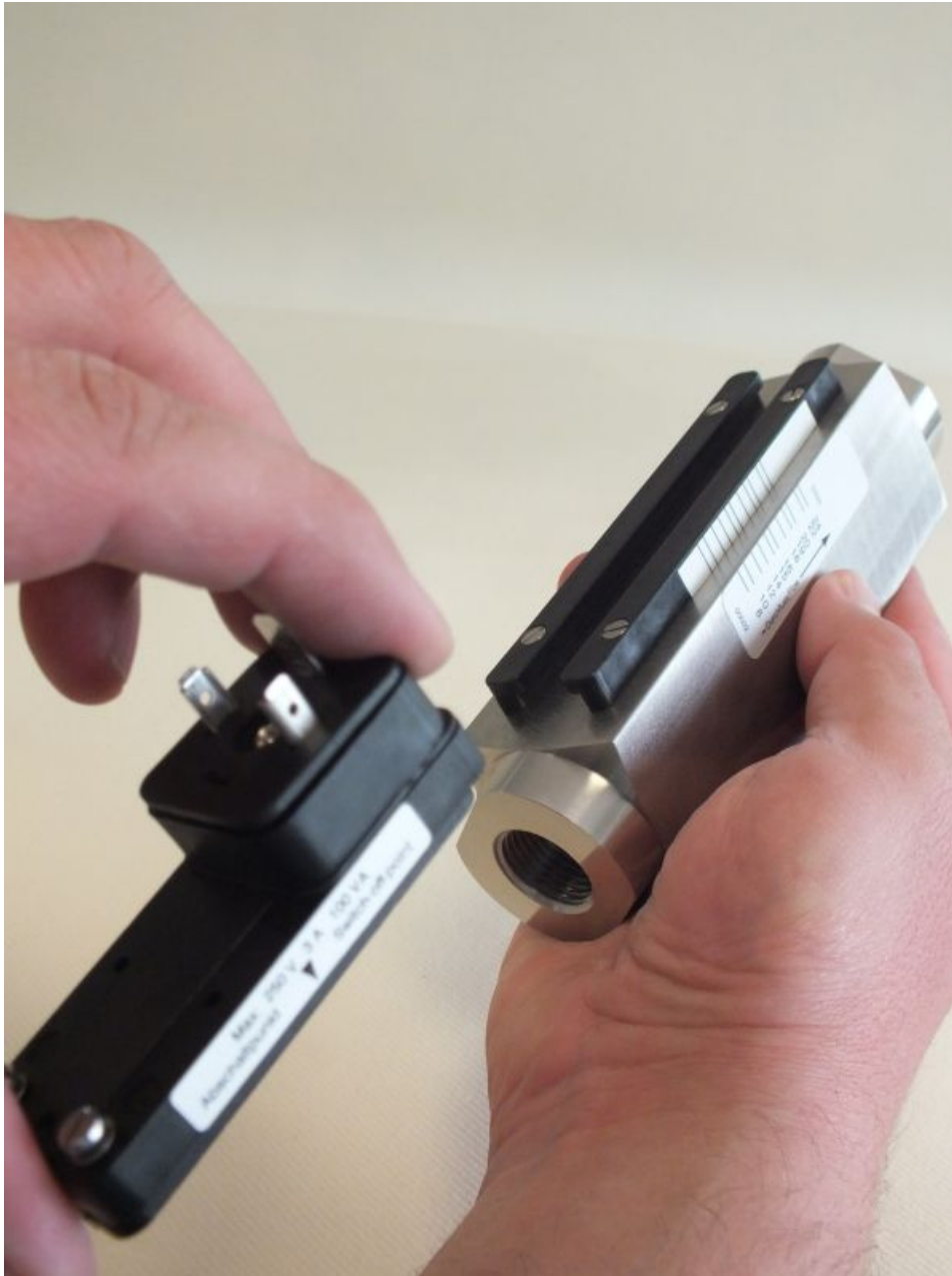
Fig. 62: Remove switch contact
