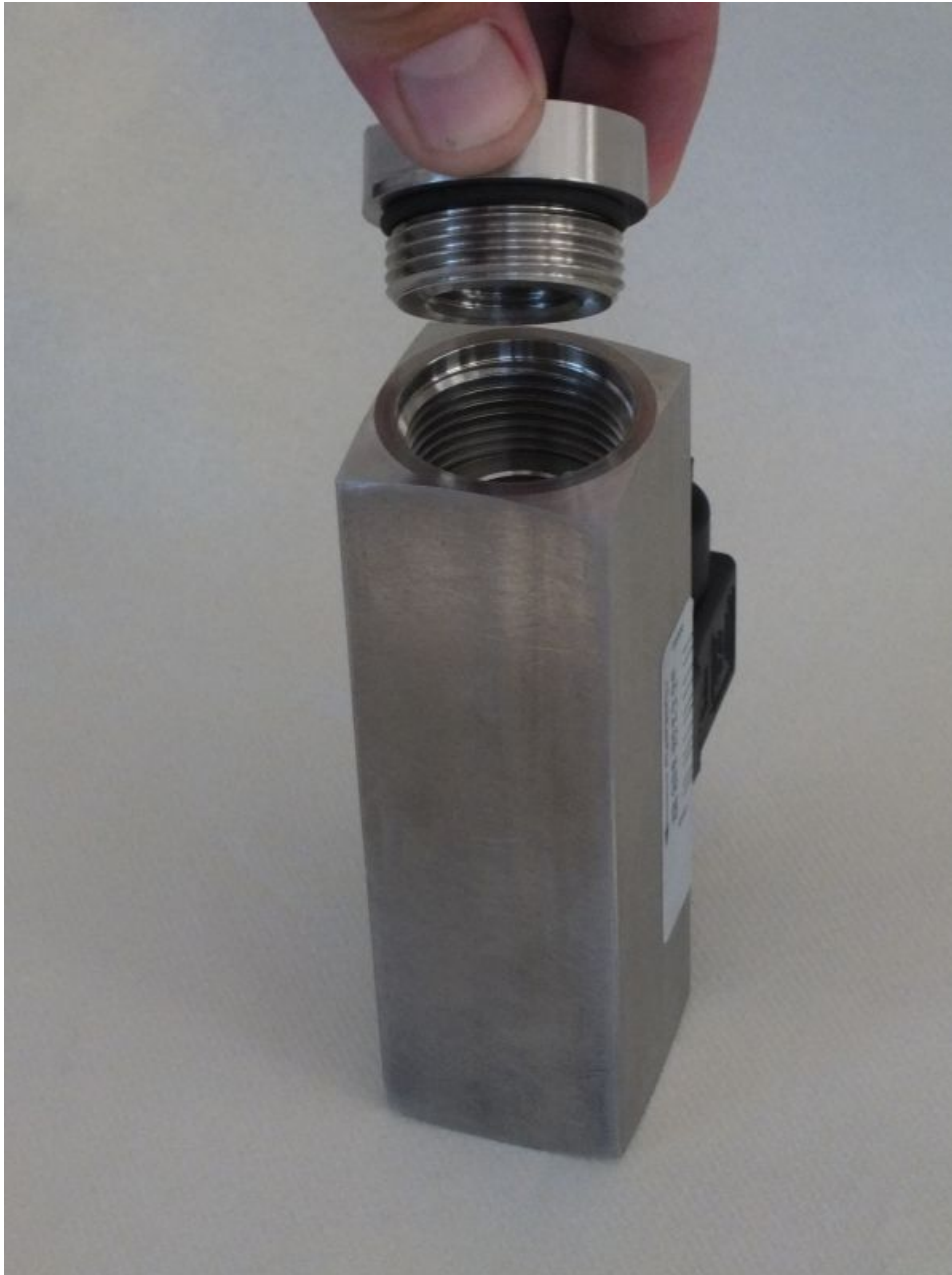
Fig. 57: Insert process connection (inlet)
