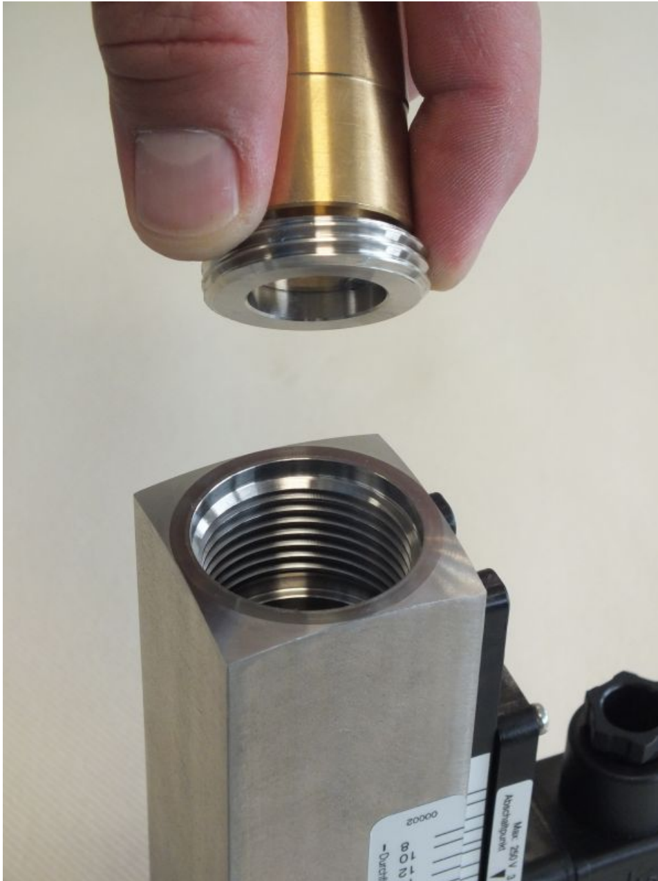
Fig. 52: Remove threaded ring (inlet)
