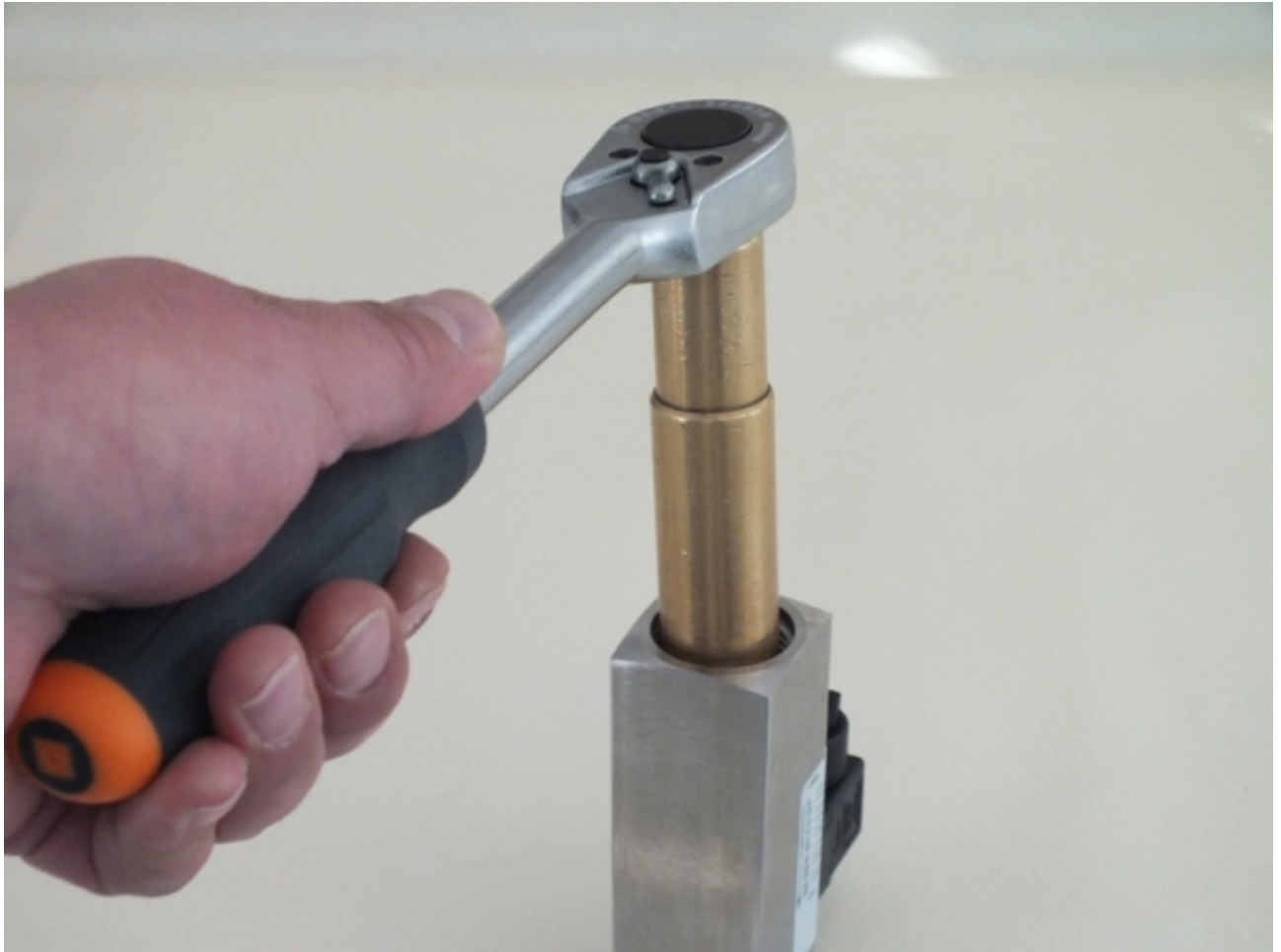
Fig. 51: Loosen threaded ring (inlet)
