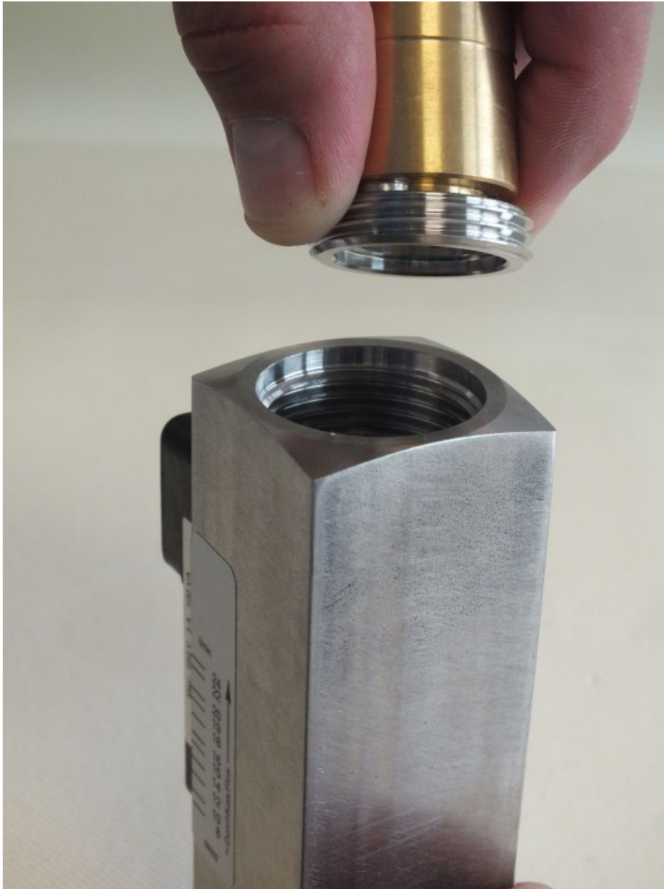
Fig. 45: Remove threaded ring (outlet)
