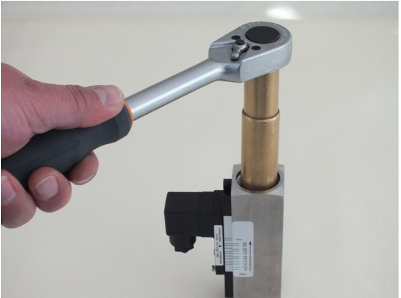
Fig. 44: Loosen threaded ring (outlet)
