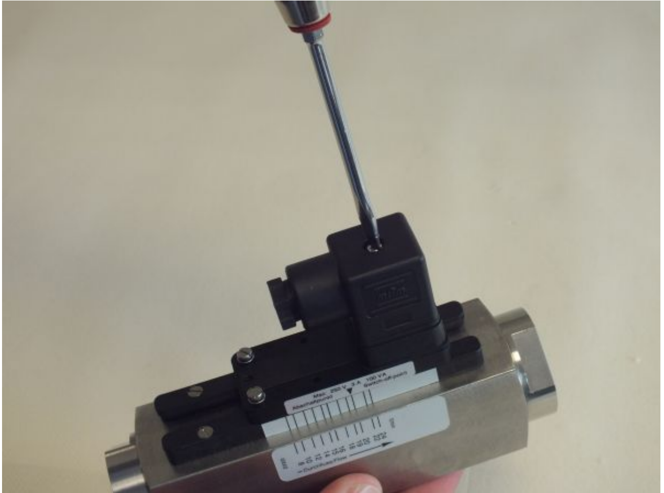
Fig. 66: Loosen female socket
