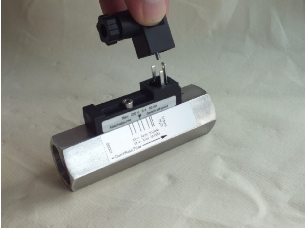
Fig. 56: Remove the female socket
