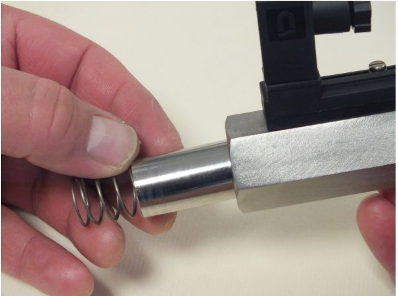
Fig. 40: Remove inner parts
