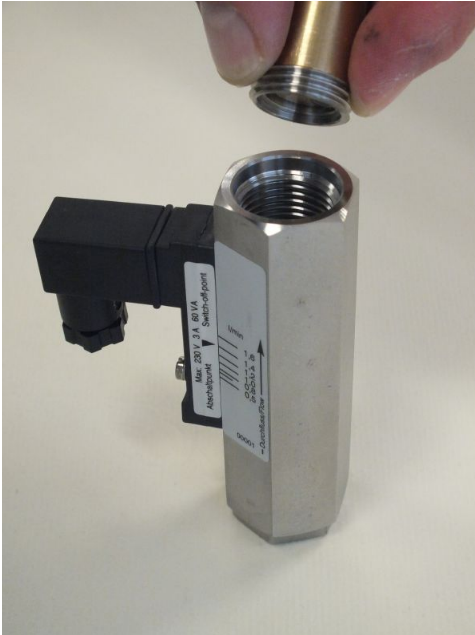
Fig. 39: Remove threaded ring (outlet)
