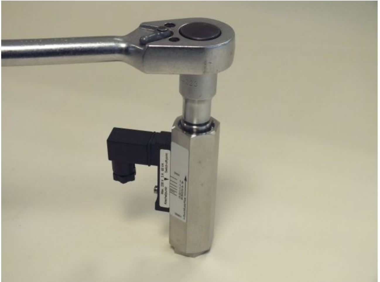
Fig. 38: Loosen threaded ring (outlet)
