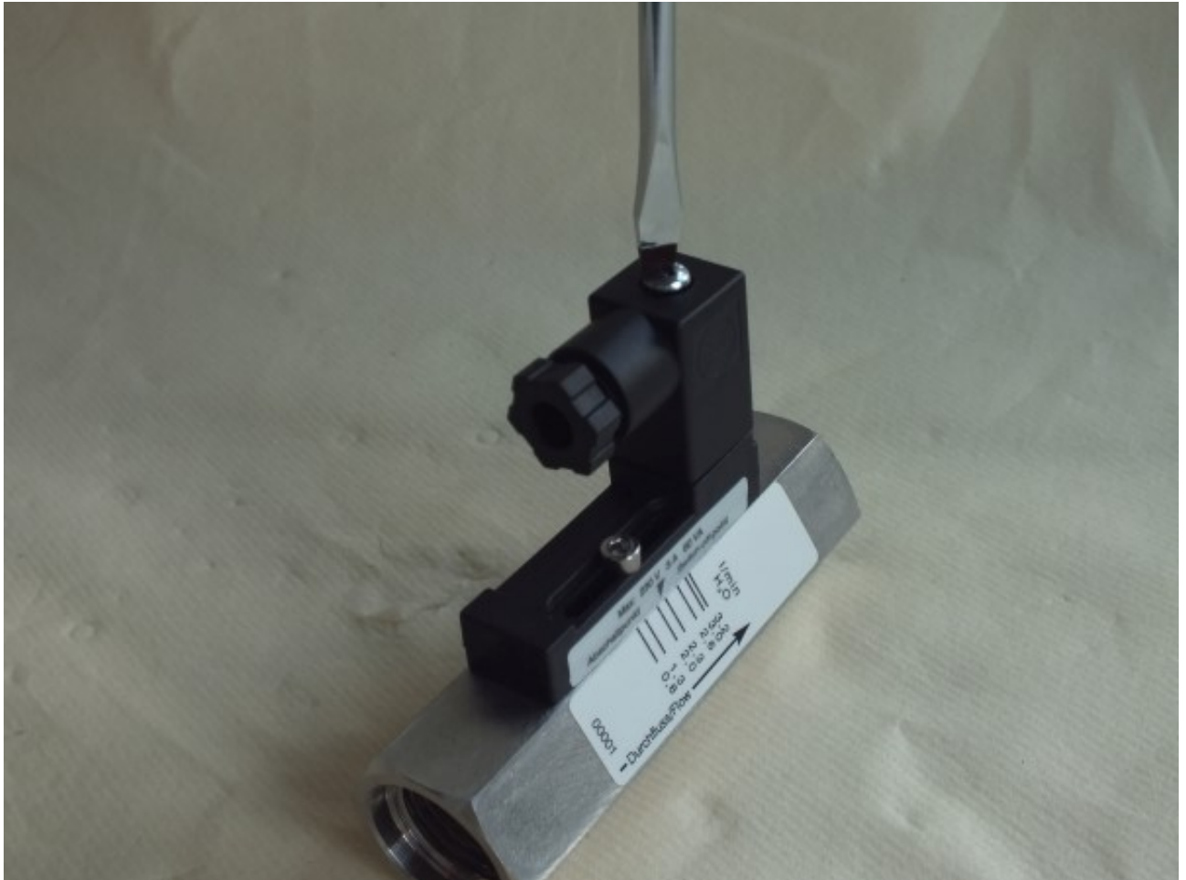
Fig. 55: Loosen female socket
