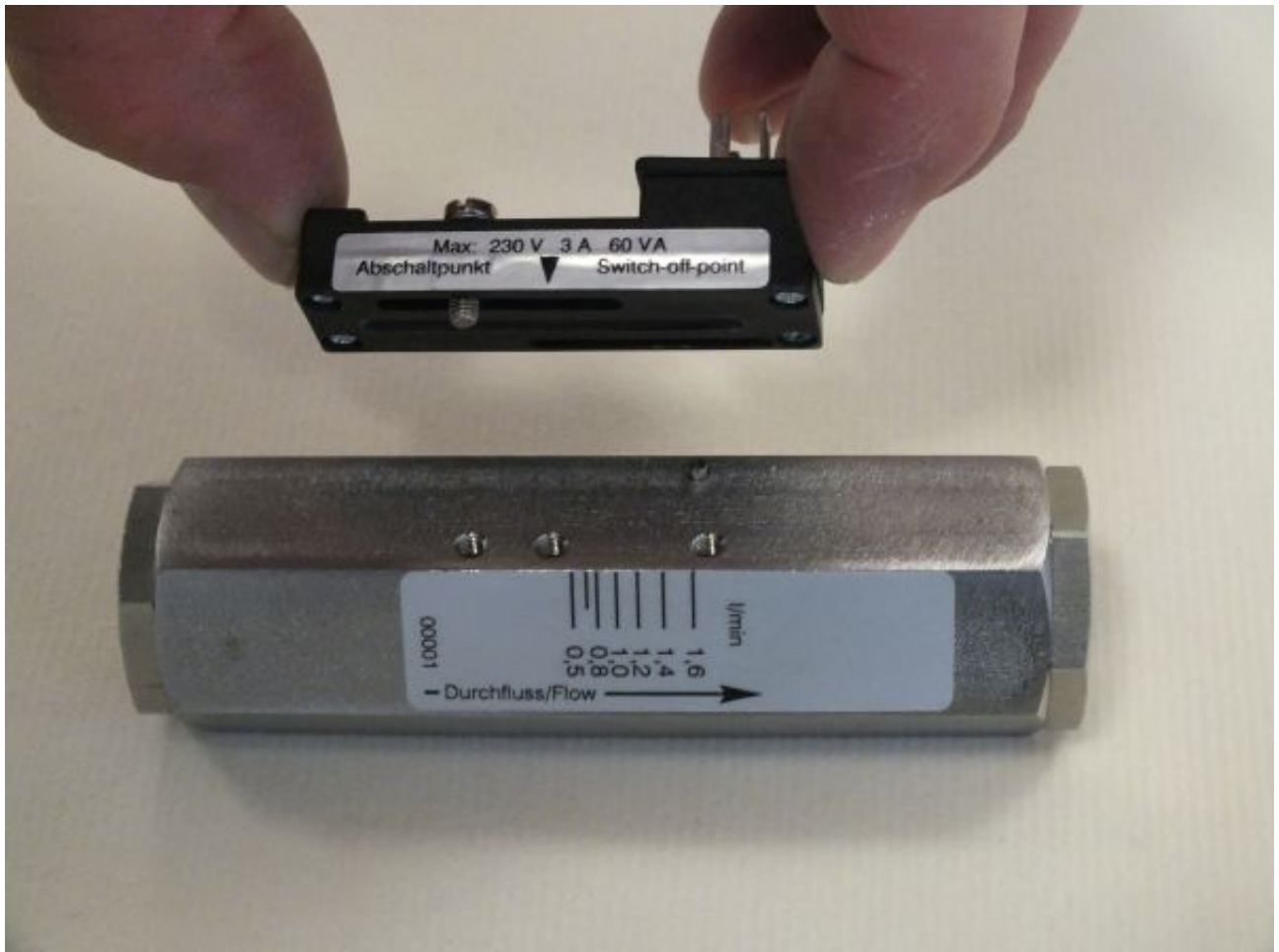
Fig. 58: Remove switch contact
