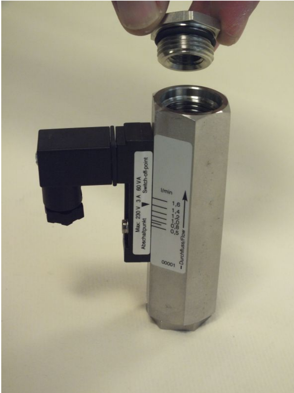
Fig. 36: Remove the process connection (outlet)
