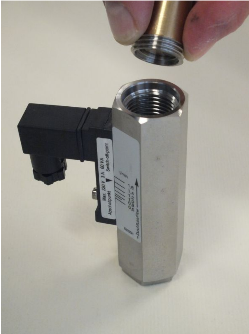
Fig. 50: Insert threaded ring (outlet)
