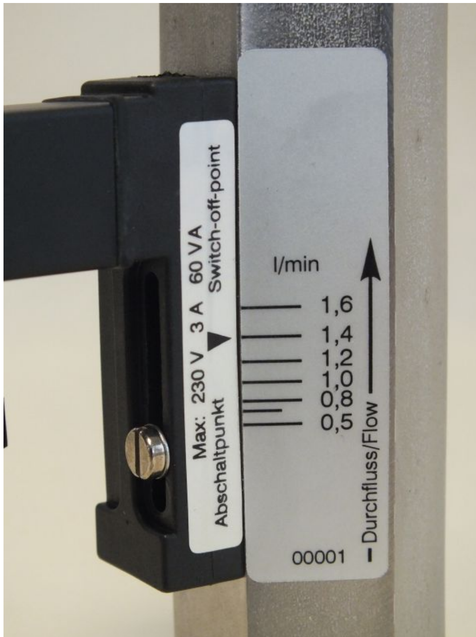
Fig. 4: Switch point adjustment scale DKM-2
