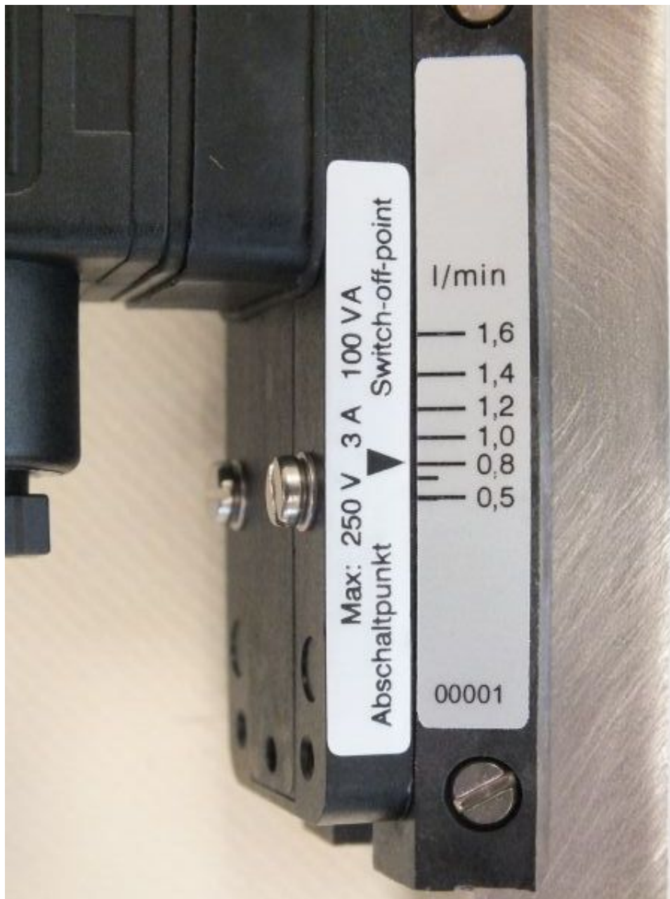
Fig. 4: Switch point adjustment scale DKM-2 30x70
