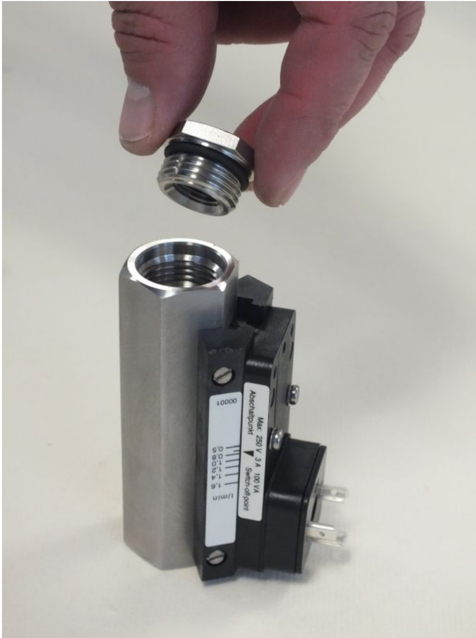
Fig. 47: Remove the process connection (inlet)
