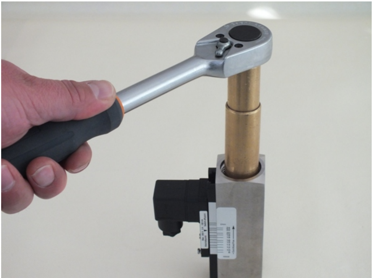
Fig. 62: Seat threaded ring (outlet)
