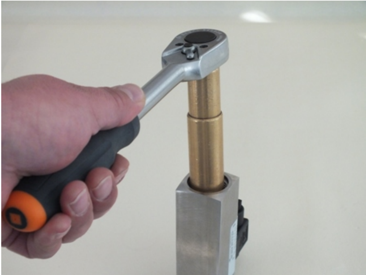
Fig. 56: Seat threaded ring (inlet)
