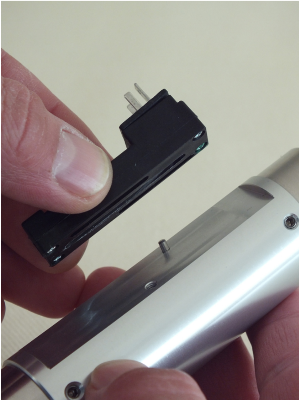
Fig. 56: Remove switch housing
