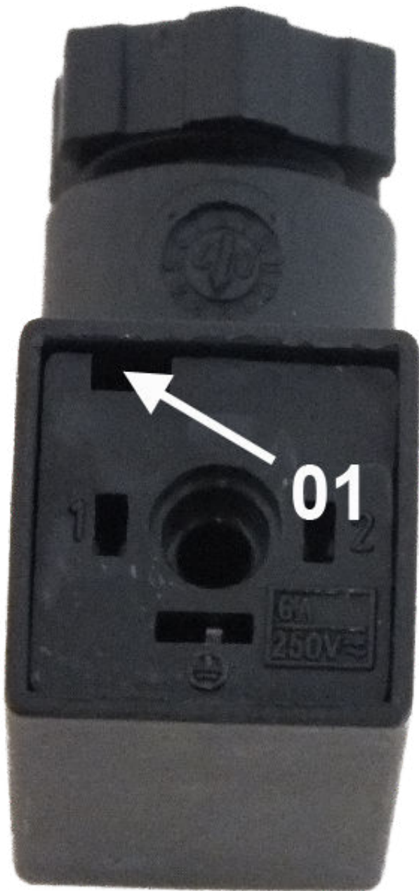
Fig. 23: Disconnect inner section
