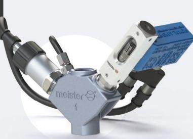
FlowBase® is an additive manufactured, tailor-made distribution system for liquid media. The FlowBase® body is developed according to customer specifications and 3D printed, so that it is optimally adapted to the requirements of the application.
