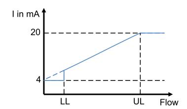
LL: Lower limit of measuring range UL: Upper limit of measuring range
