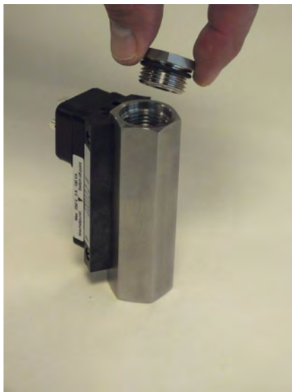
Fig. 53: Insert process connection (outlet)
