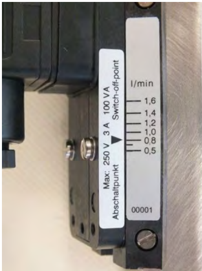
Fig. 35: Reading-off the switch point value
