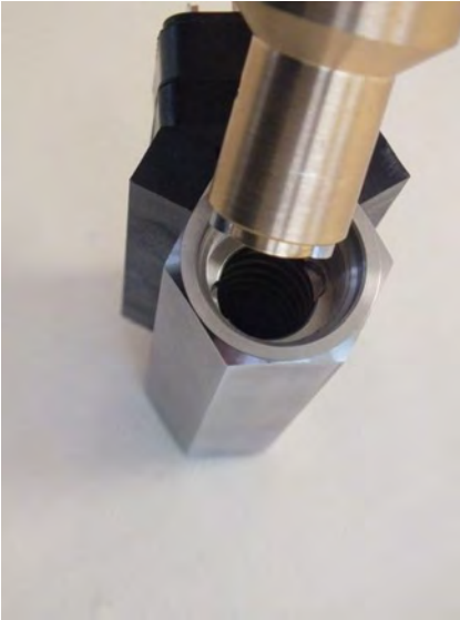
Fig. 38: Insert threaded ring insertion tool (outlet)
