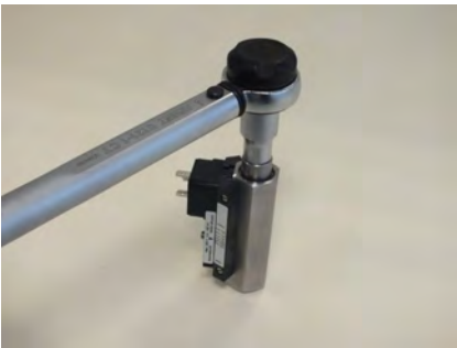
Fig. 39: Loosen threaded ring (outlet)
