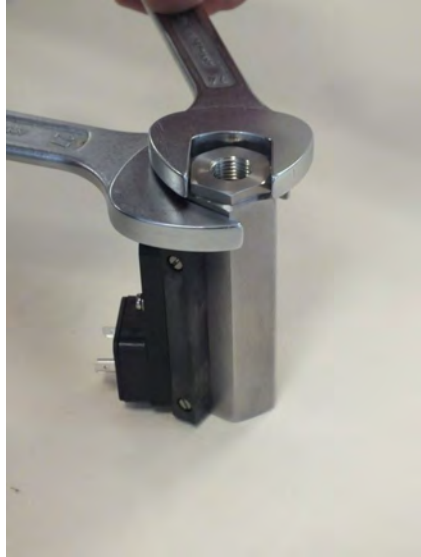
Fig. 43: Loosen process connection (inlet)
