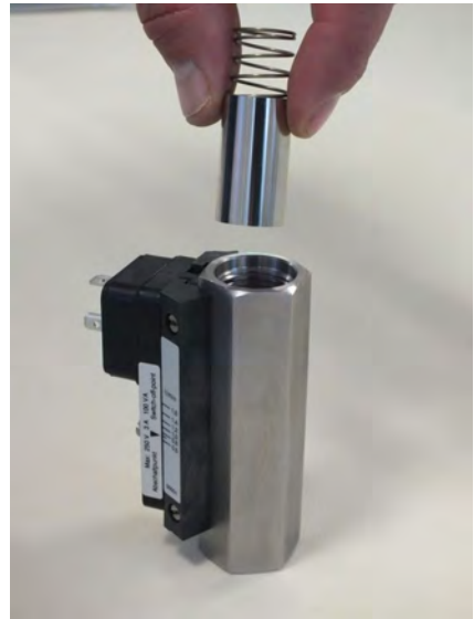
Fig. 50: Insert inner parts
