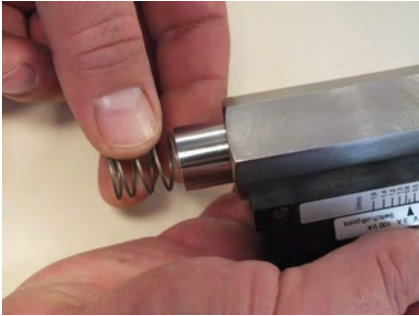
Fig. 41: Remove inner parts
