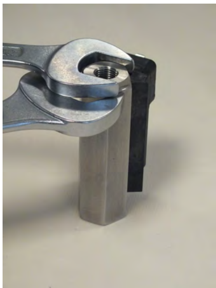
Fig. 54: Tighten process connection (outlet)
