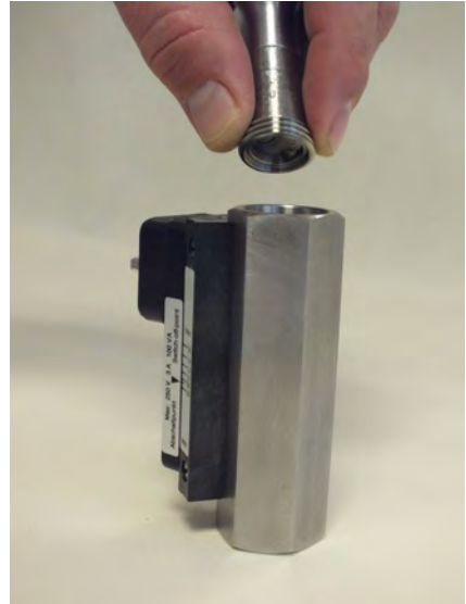
Fig. 40: Remove threaded ring (outlet)
