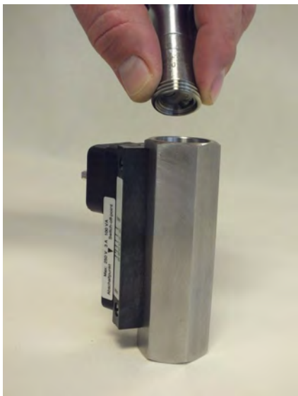
Fig. 51: Insert threaded ring (outlet)
