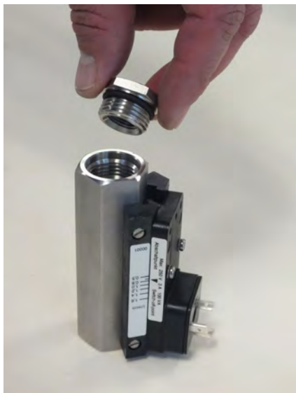
Fig. 47: Insert process connection (inlet)
