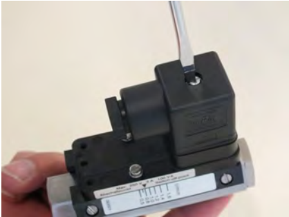
Fig. 56: Loosen female socket
