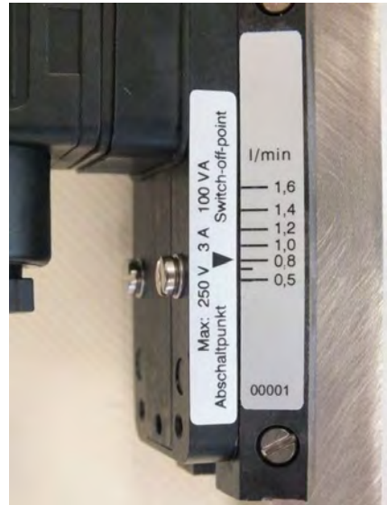
Fig. 4: Switch point adjustment scale RVM/U-2 30x70
