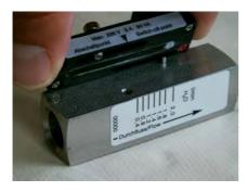
Fig. 53: Remove switch contact
