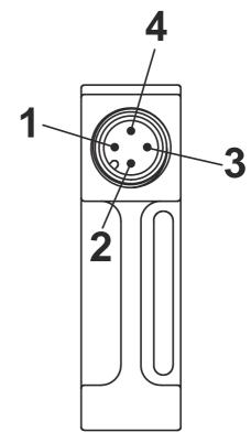
Fig. 17: Pin assignment, connector M12x1 (Form 15x50)
