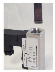
Fig. 35: Insert threaded ring insertion tool (outlet)
