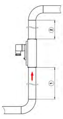
Fig. 6: Unimpeded flow sections
