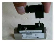
Fig. 22: Remove socket
