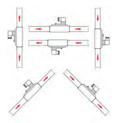
Fig. 5: Installation position/direction of flow
