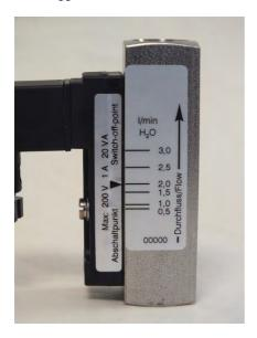
Fig. 34: Reading-off the flow value (example scale)
