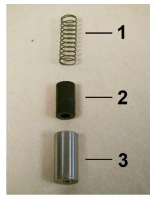
Fig. 39: Spring, magnets and float
