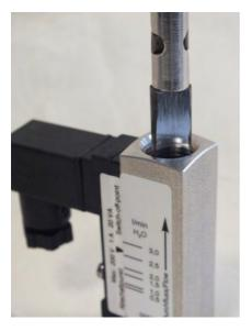
Fig. 36: Loosen threaded ring (outlet)
