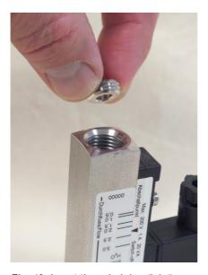
Fig. 43: Insert threaded ring (inlet)
