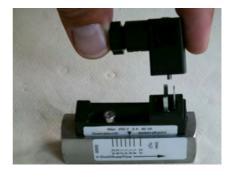
Fig. 51: Remove female socket
