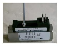
Fig. 52: Loosen set screw
