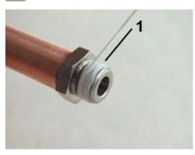
Fig. 9: Apply sealing thread
