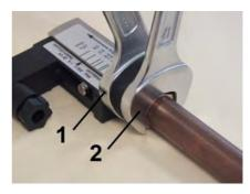
Fig. 11: Screw in the device
