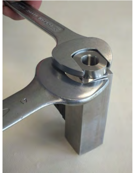
Fig. 59: Tighten process connection (inlet)
