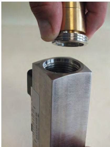
Fig. 46: Remove threaded ring (outlet)
