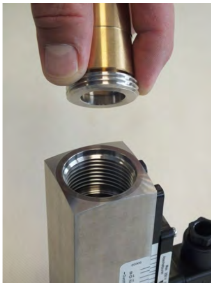
Fig. 53: Remove threaded ring (inlet)
