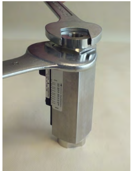
Fig. 42: Loosen process connection (outlet)
