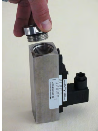
Fig. 50: Remove the process connection (inlet)
