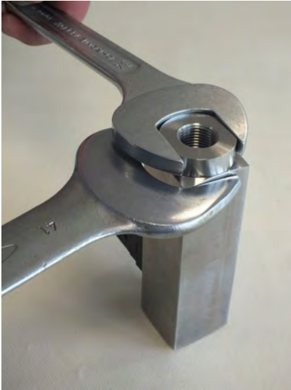
Fig. 49: Loosen process connection (inlet)
