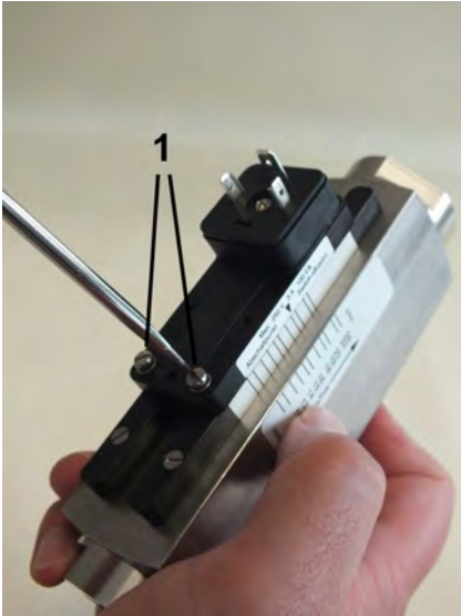
Fig. 74: Loosen set screws
