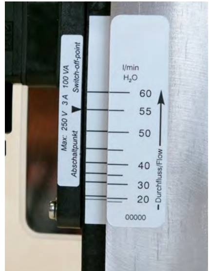
Fig. 4: Switch point adjustment scale
