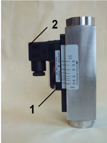
Fig. 3: Switch contact and female socket
