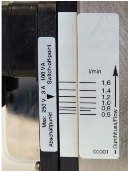
Fig. 35: Reading-off the flow value
