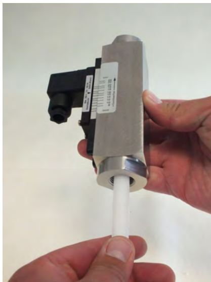
Fig. 66: Check for smooth operation
