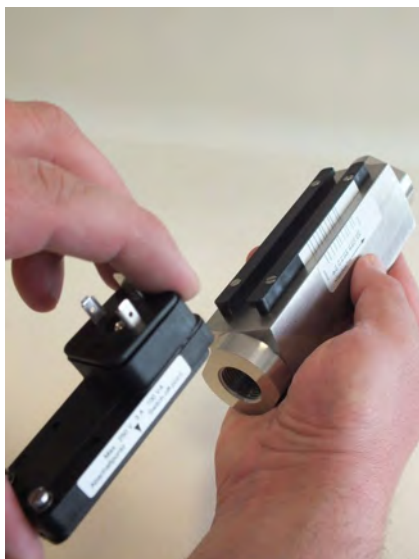
Fig. 76: Remove switch contact
