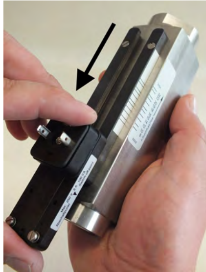
Fig. 75: Remove switch contact from guide rails
