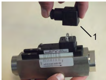
Fig. 73: Remove female socket
