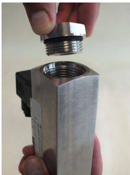
Fig. 64: Insert process connection (outlet)
