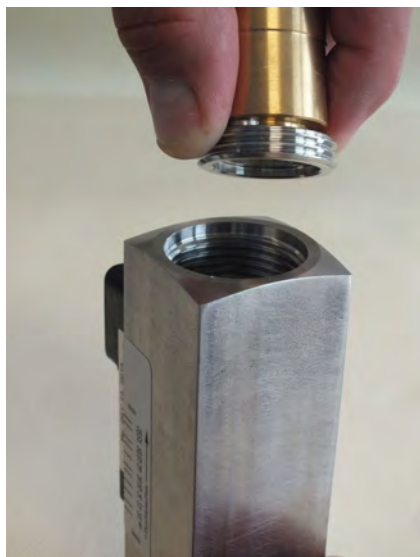
Fig. 62: Insert threaded ring (outlet)
