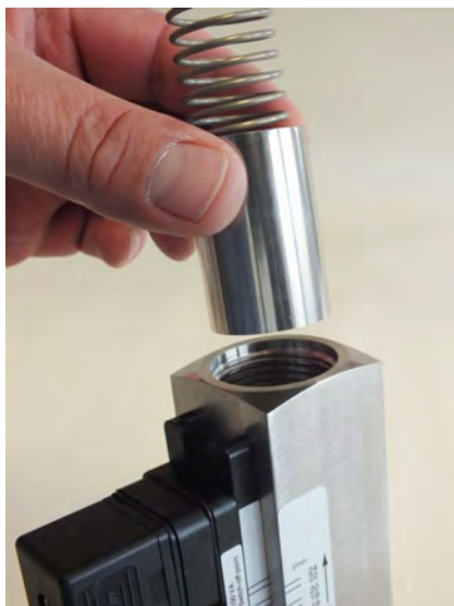
Fig. 61: Insert inner parts
