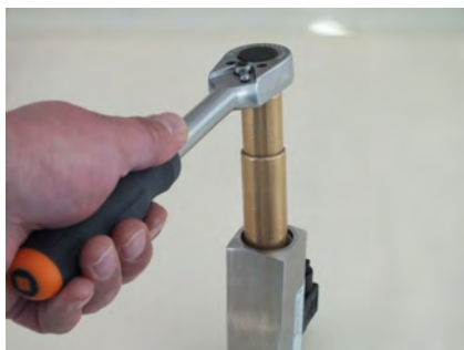
Fig. 52: Loosen threaded ring (inlet)
