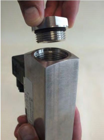
Fig. 37: Remove the process connection (outlet)
