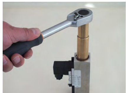
Fig. 39: Loosen threaded ring (outlet)
