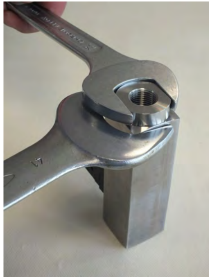
Fig. 53: Tighten process connection (inlet)
