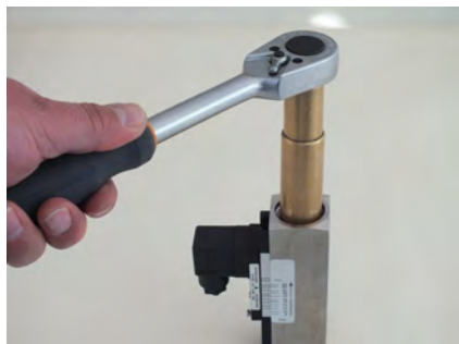
Fig. 57: Seat threaded ring (outlet)
