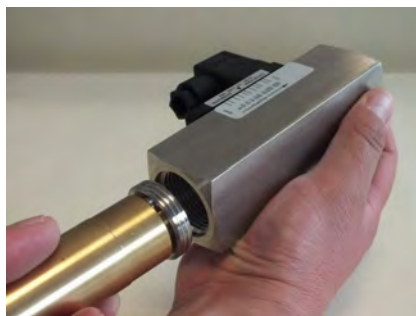
Fig. 50: Insert threaded ring (inlet)
