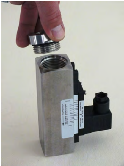
Fig. 52: Insert process connection (inlet)
