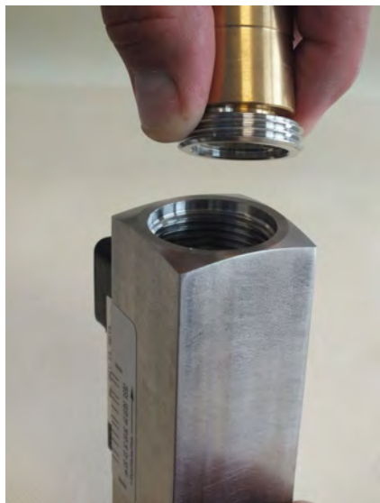
Fig. 56: Insert threaded ring (outlet)
