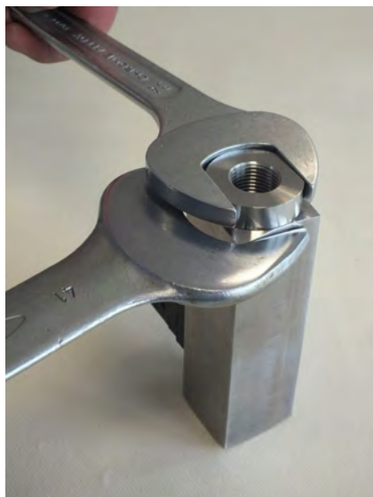
Fig. 43: Loosen process connection (inlet)
