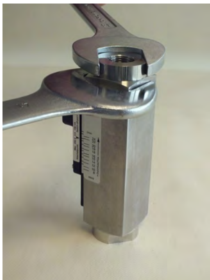
Fig. 59: Tighten process connection (outlet)
