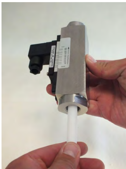
Fig. 60: Check for smooth operation
