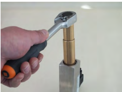
Fig. 46: Loosen threaded ring (inlet)
