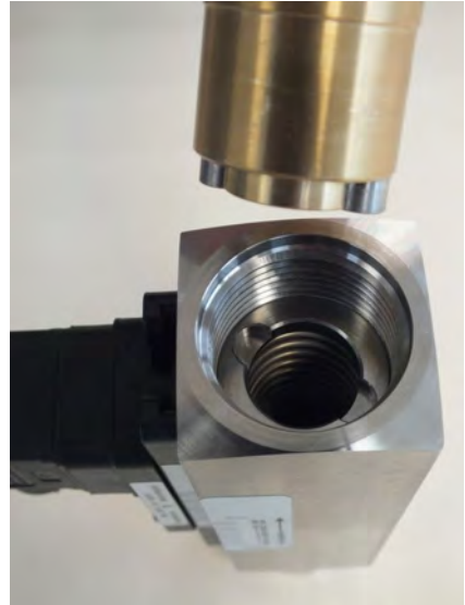
Fig. 38: Insert threaded ring insertion tool (outlet)
