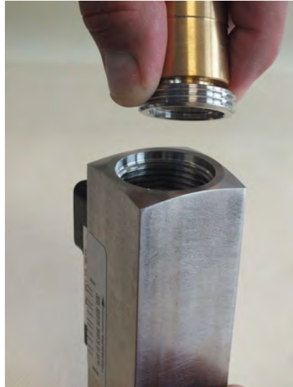
Fig. 47: Remove threaded ring (inlet)
