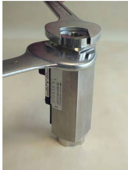
Fig. 36: Loosen process connection (outlet)
