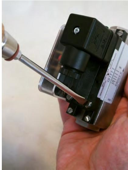
Fig. 69: Loosen set screws
