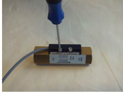
Fig. 32: Loosen set screws
