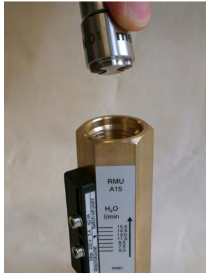
Fig. 22: Insert threaded ring insertion tool (outlet)
