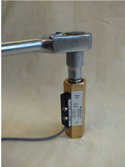
Fig. 23: Loosen threaded ring (outlet)
