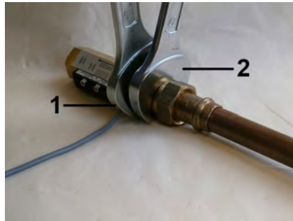
Fig. 12: Screw in the device
