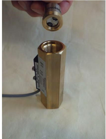
Fig. 24: Remove threaded ring (outlet)
