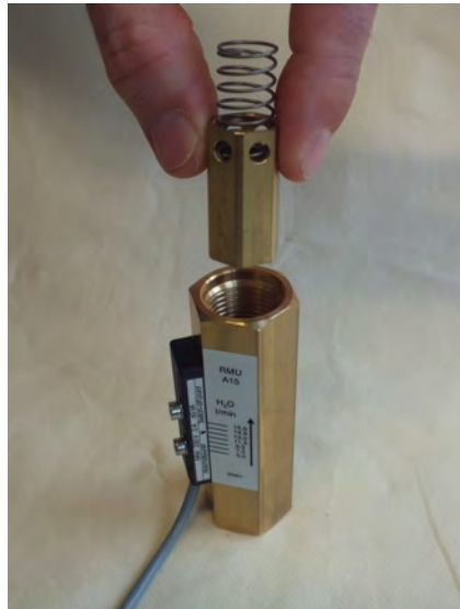
Fig. 28: Insert inner parts
