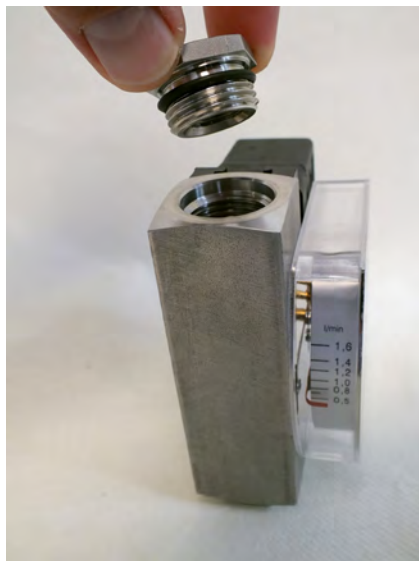
Fig. 60: Insert process connection (outlet)
