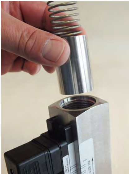
Fig. 57: Insert inner parts
