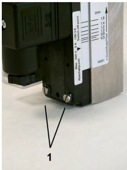
Fig. 34: Loosen set screws
