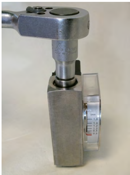
Fig. 46: Loosen threaded ring (outlet)
