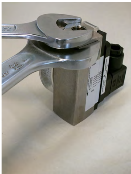
Fig. 55: Tighten process connection (inlet)
