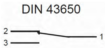
Fig. 16: Switch position under no-flow condition
