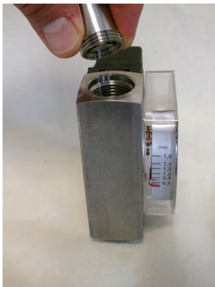
Fig. 47: Remove threaded ring (outlet)
