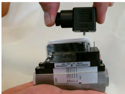
Fig. 69: Remove female socket
