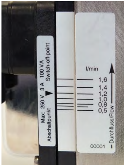
Fig. 36: Reading-off the flow value
