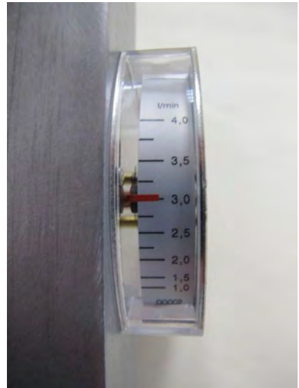
Fig. 37: Reading-off the display value
