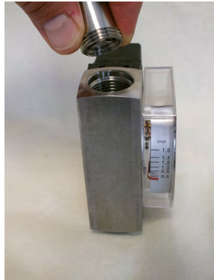
Fig. 58: Insert threaded ring (outlet)
