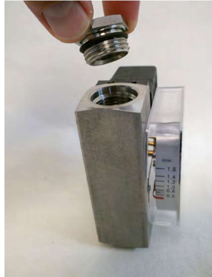
Fig. 44: Remove the process connection (outlet)
