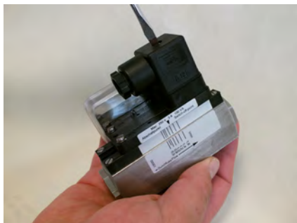
Fig. 68: Loosen female socket
