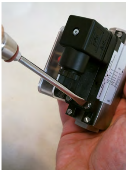
Fig. 70: Loosen set screws
