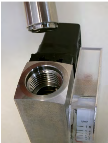
Fig. 45: Insert threaded ring insertion tool (outlet)
