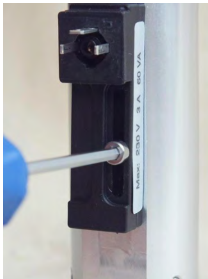
Fig. 32: Loosen set screw
