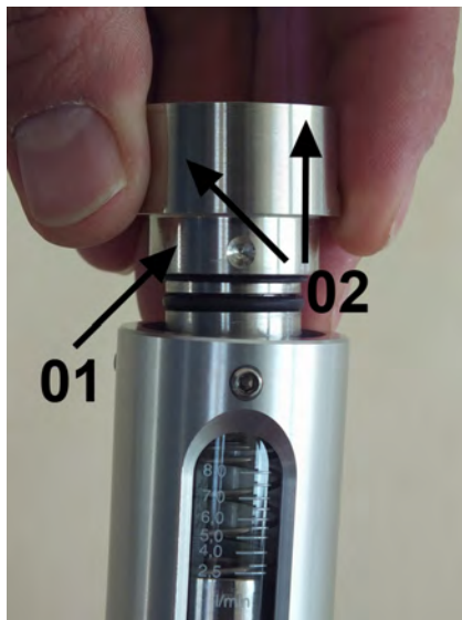
Fig. 50: Position process connection (outlet) in device housing
