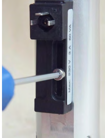
Fig. 33: Loosen set screw
