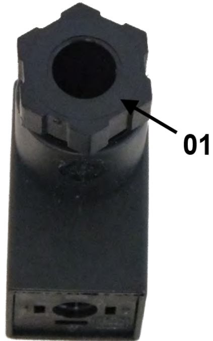
Fig. 24: Disconnect the screw connection
