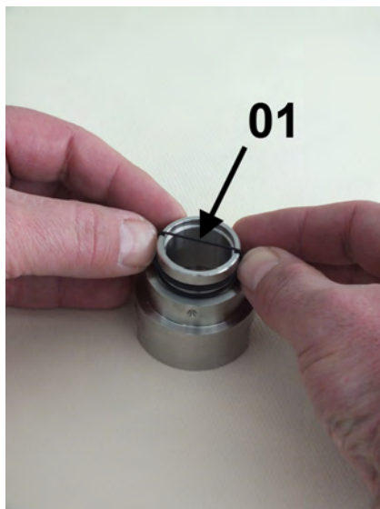
Fig. 41: O-ring (Glass buffer)
