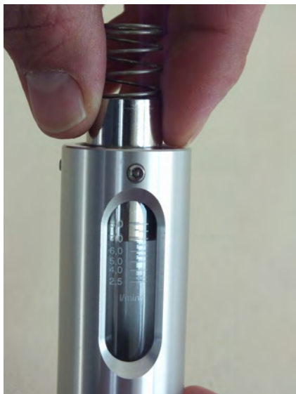
Fig. 49: Insert float and inner parts
