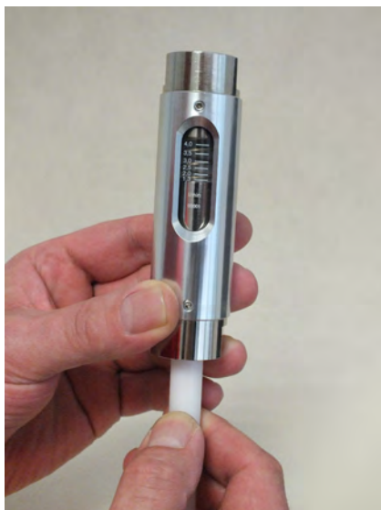
Fig. 52: Check for ease of movement
