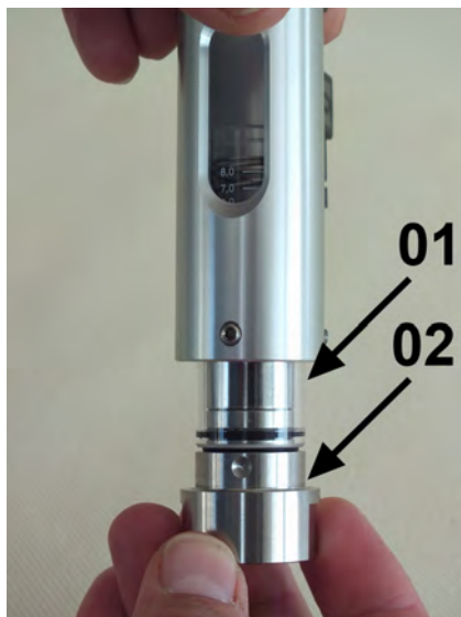
Fig. 38: Remove the inner section
