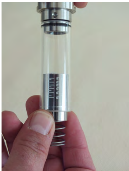
Fig. 39: Remove float, magnets and spring
