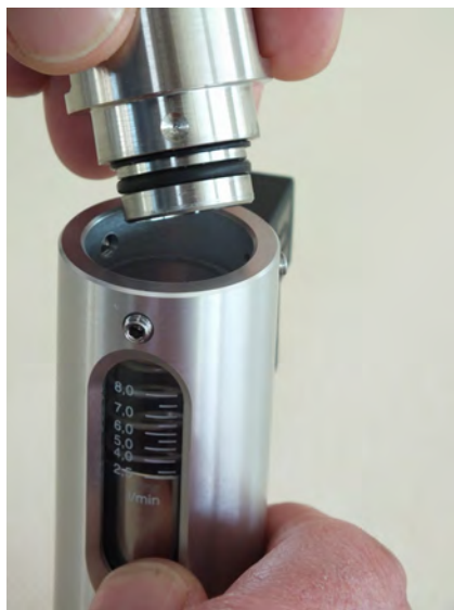
Fig. 36: Remove the process connection (outlet)
