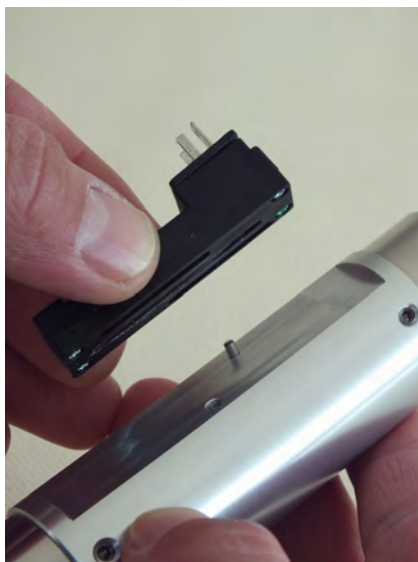
Fig. 56: Remove switch housing
