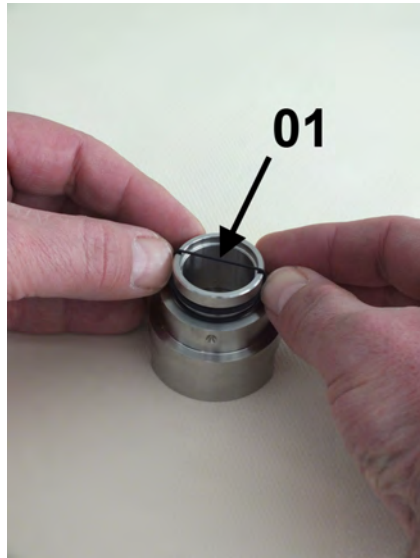
Fig. 42: O-ring (Glass buffer)
