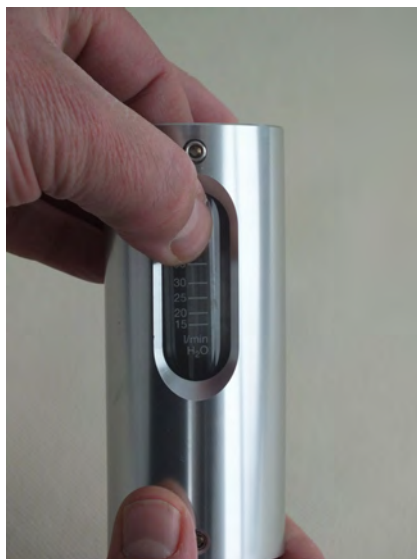
Fig. 49: Align the sight glass
