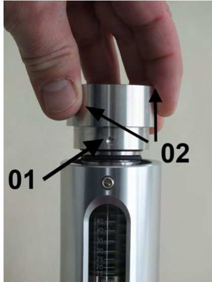
Fig. 51: Position process connection (outlet) in device housing
