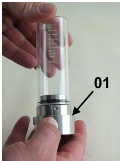
Fig. 45: Process connection (inlet) in sight glass
