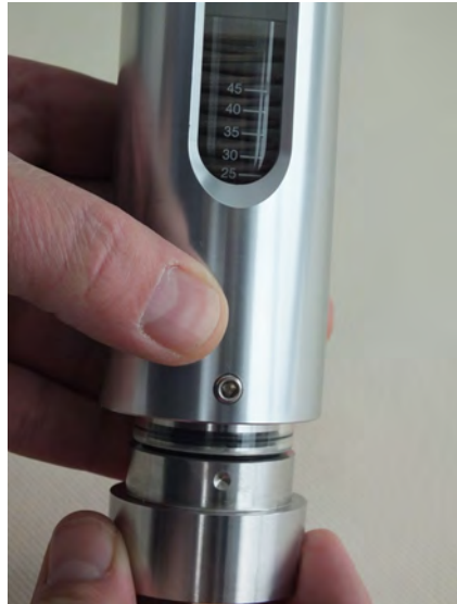
Fig. 47: Insert the process connection into the device housing
