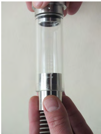
Fig. 40: Remove float, magnets and spring
