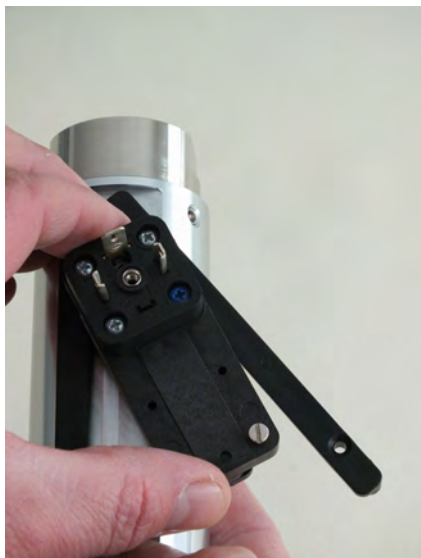
Fig. 58: Rotate guide rail to the side
