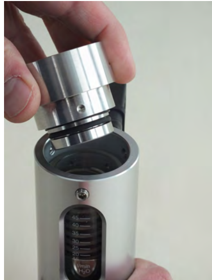
Fig. 37: Remove the process connection (outlet)
