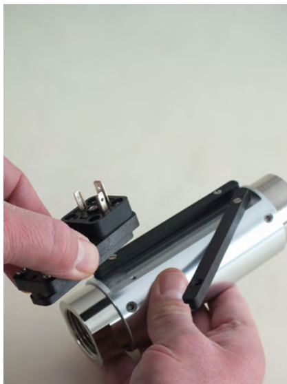
Fig. 59: Remove switch contact
