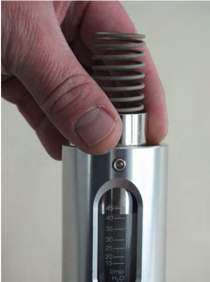
Fig. 50: Insert float and inner parts
