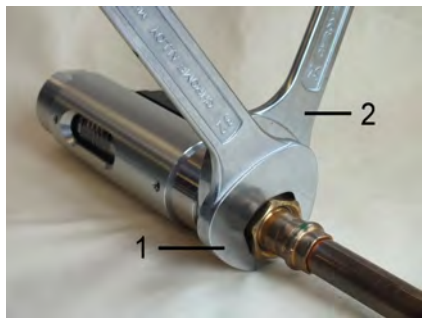
Fig. 11: Screw in the device
