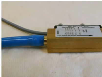
Fig. 10: Hose connected to device
