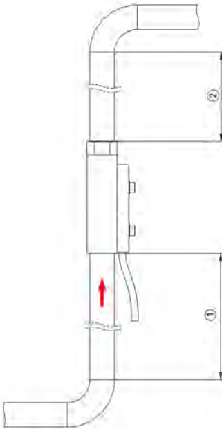
Fig. 6: Unimpeded flow sections
