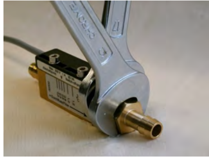
Fig. 29: Tighten process connection (outlet)
