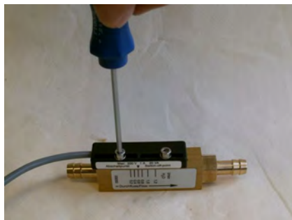
Fig. 31: Loosen set screws
