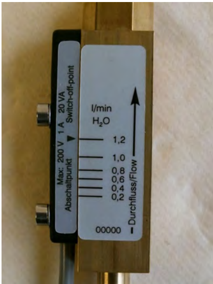
Fig. 19: Reading-off the flow value (example switch point adjustment scale)
