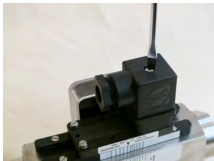
Fig. 64: Loosen female socket
