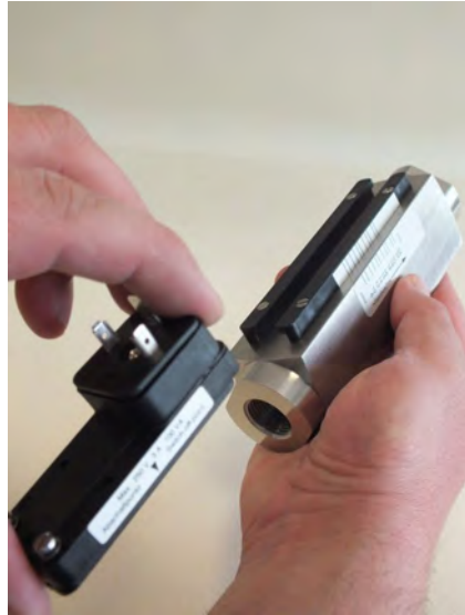
Fig. 68: Remove switch contact
