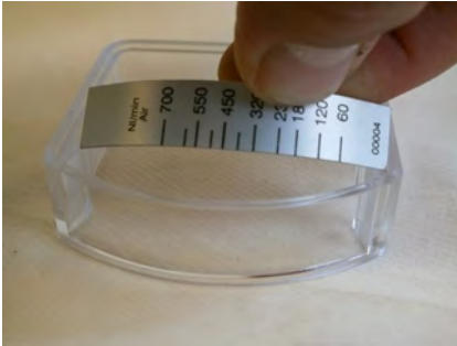
Fig. 40: Removal of the scale support
