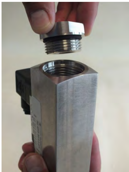
Fig. 56: Insert process connection (outlet)
