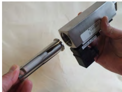
Fig. 45: Remove inner parts
