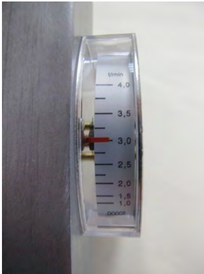
Fig. 36: Read-off display value (example)
