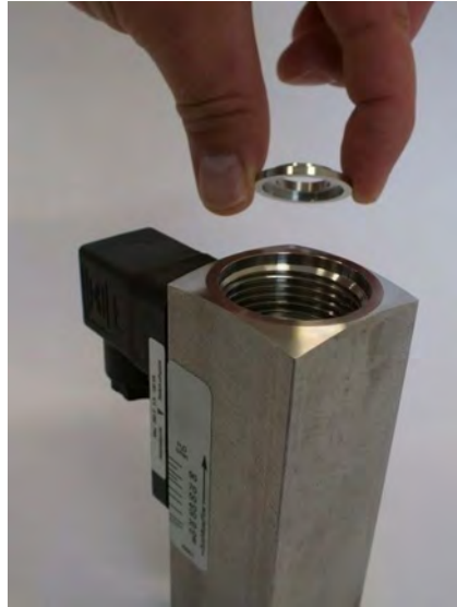
Fig. 44: Remove the centering disc (outlet)
