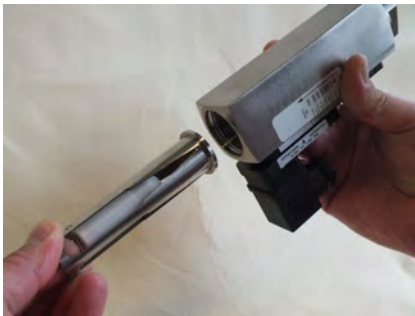
Fig. 54: Insert inner parts
