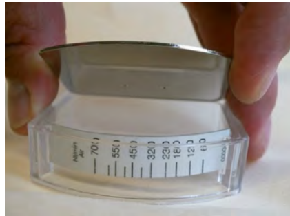
Fig. 39: Removal of display cover plate from housing
