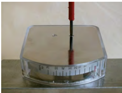
Fig. 39: Removal of display cover plate from housing
