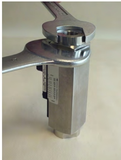
Fig. 35: Loosen process connection (outlet)
