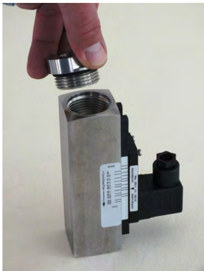
Fig. 44: Insert process connection (inlet)
