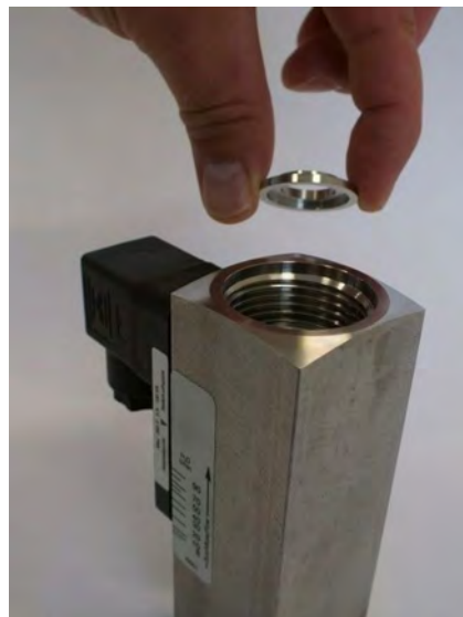
Fig. 48: Insert centering disc (outlet)
