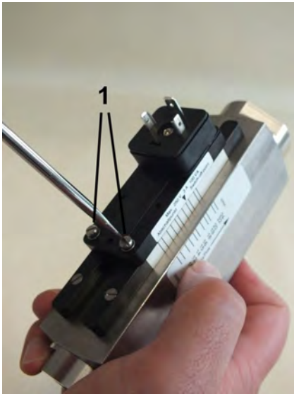
Fig. 54: Loosen set screws
