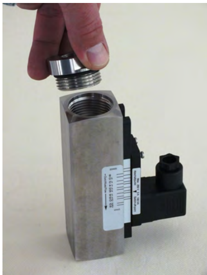
Fig. 41: Remove the process connection (inlet)
