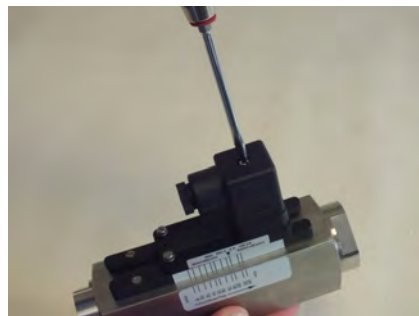
Fig. 52: Loosen female socket
