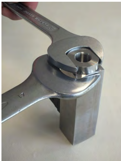
Fig. 45: Tighten process connection (inlet)
