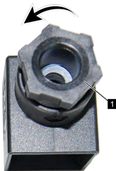
Fig. 24: Loosen the screw connection
