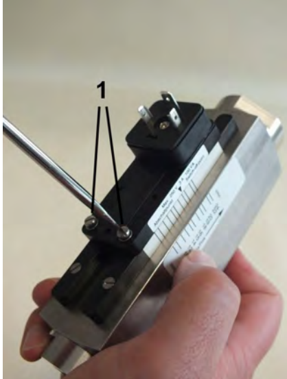
Fig. 33: Loosen the set screws
