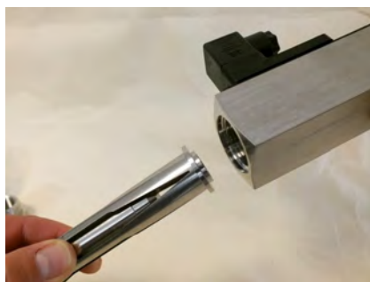
Fig. 38: Remove inner parts
