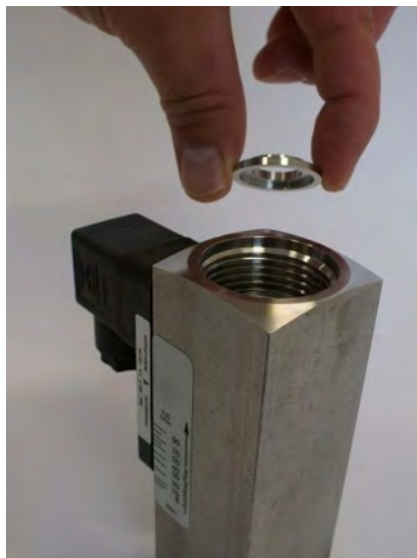
Fig. 37: Remove the centering disc (outlet)
