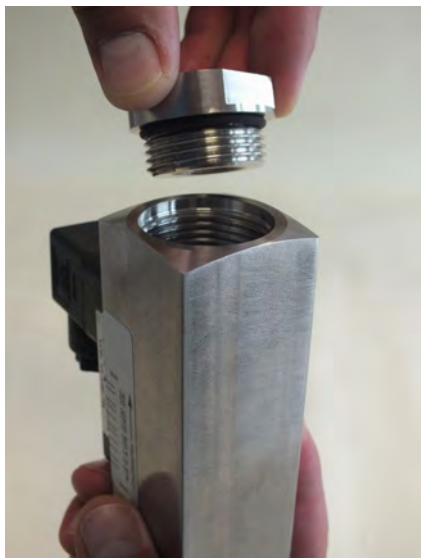
Fig. 49: Insert process connection (outlet)
