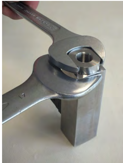
Fig. 40: Loosen process connection (inlet)
