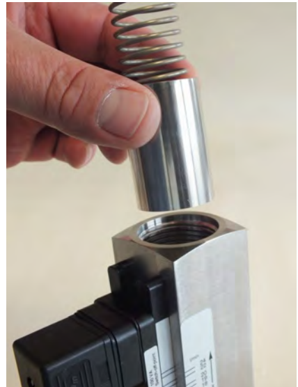
Fig. 55: Insert inner parts
