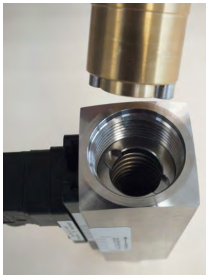
Fig. 38: Insert threaded ring insertion tool (outlet)
