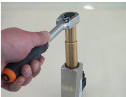
Fig. 46: Loosen threaded ring (inlet)
