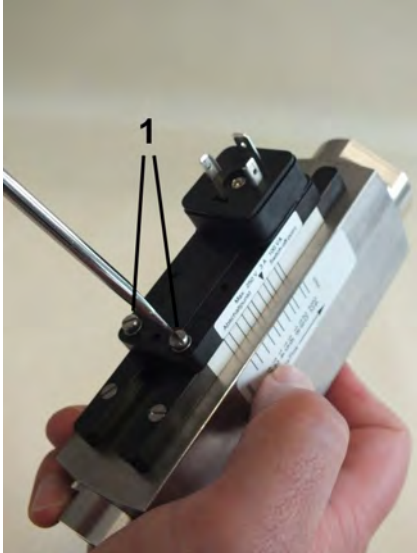
Fig. 34: Loosen the set screws
