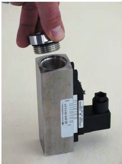
Fig. 44: Remove the process connection (inlet)
