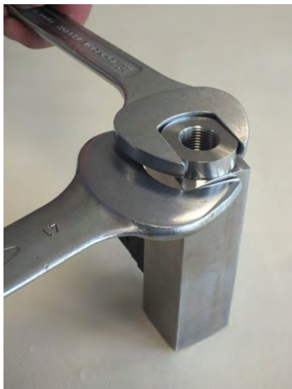
Fig. 43: Loosen process connection (inlet)
