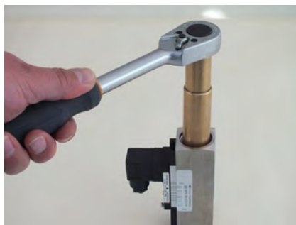
Fig. 39: Loosen threaded ring (outlet)
