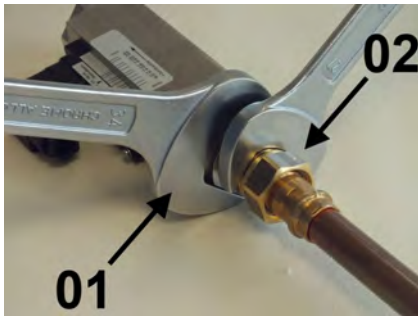
Fig. 11: Screw in the device
