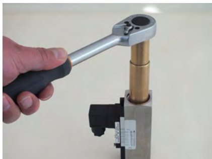
Fig. 57: Seat threaded ring (outlet)
