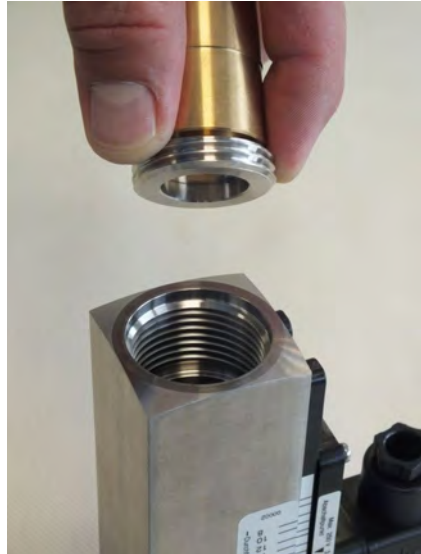
Fig. 47: Remove threaded ring (inlet)
