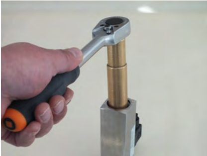
Fig. 51: Seat threaded ring (inlet)
