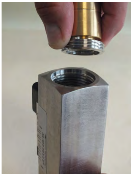
Fig. 56: Insert threaded ring (outlet)
