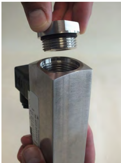
Fig. 58: Insert process connection (outlet)
