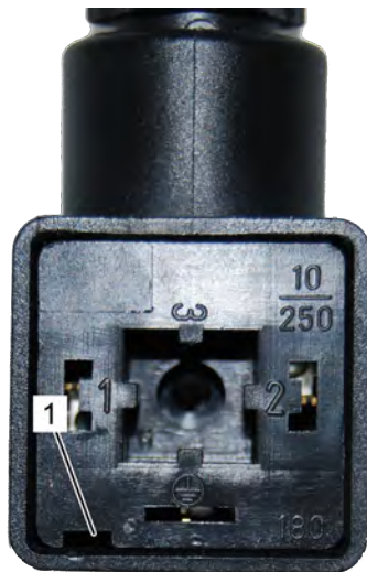
Fig. 24: Disconnect inner section
