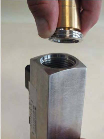
Fig. 40: Remove threaded ring (outlet)
